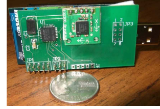
Figure 2. The sensor board with the accelerometer and gyroscope. The mother board at the back is Tmote Sky.
