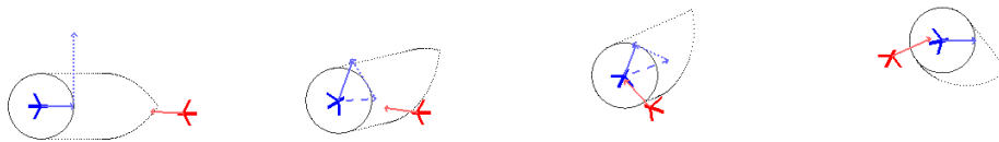
Figure 8: Evader keeps pursuer from entering reachable set, and hence avoids collision (animation at [60])
