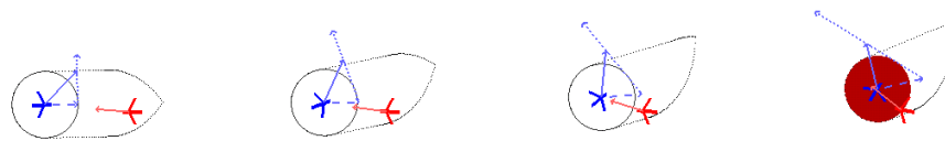
Figure 9: Pursuer starts within the reachable set, and can thus cause a collision despite the evader's efforts (animation at [60])
