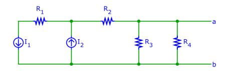
14. Find algebraic expressions for the circuit elements of a Thévenin equivalent circuit representing the behavior at terminals a-b of the circuit shown below.
