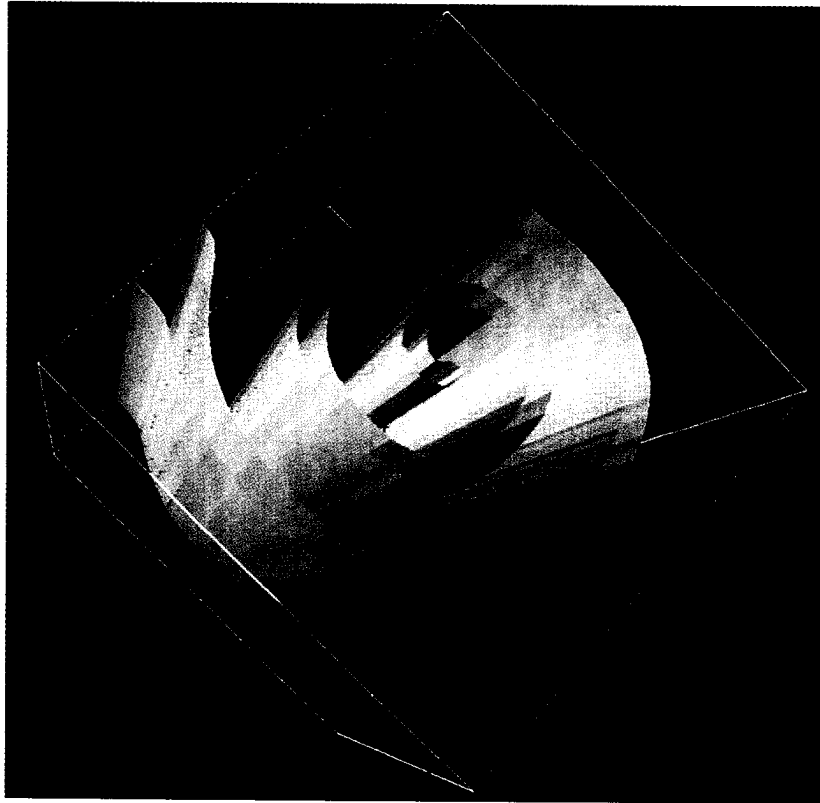
Fig. 8. Isosurfaces for a straight scroll wave, generated from a 48 \times 48 \times 48 array of Chua's circuits. Here, as well as in all subsequent figures, the isosurfaces correspond to the level -1.503 of variable x .
