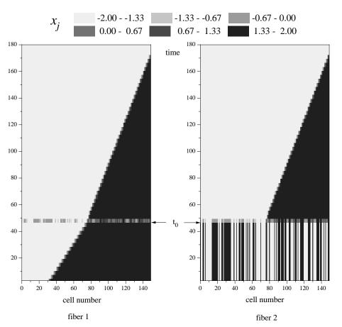
**Fig. 4.** Propagation failure overcomed in coupled *bistable* fibers. Diffusion coefficients:  $D_1 = 3$ ,  $D_2 = 0.2$ . At  $t_0 = 48$  the inter-fiber interaction is switched-on, h = 10. Vertical axes account for time in arbitrary units (a.u.).
