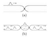
Fig. 7. Schematic diagram of two parallel fibers coupled by (a) a single-pin contact and (b) a double-pin contact.
