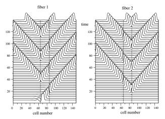
Fig. 9. A generator of synchronized pulses when the parallel excitable fibers have two-pin contacts. Parameter values:  $\alpha = 4.5$ , D = 2,  $h_{65} = h_{85} = 5$ . Vertical axes account for time in arbitrary units (a.u.).
