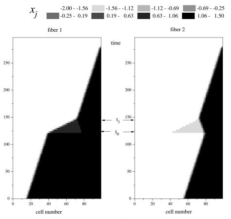
Fig. 2. Wave fronts in two identical bistable fibers with D = 2. (a) Synchronization of two wave fronts traveling with finite time delay. For  $t < t_0 = 120$  the chains are independent, h = 0. At  $t = t_0$ , the interaction is switched-on,  $t > t_0$ , h = 0.5. The time interval  $t_0 < t < t_1 \approx 140$  corresponds to a transient process. Vertical axes account for time in arbitrary units (a.u.).
