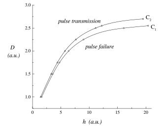
Fig. 8. Diagram of pulse driving by single-pin contact in (D, h) parameter plane. The pulse fails to propagate for values chosen below the curve  $C_1$ . Above the curve  $C_2$  the pulse successfully overcomes the contact. Units are arbitrary (a.u.).
