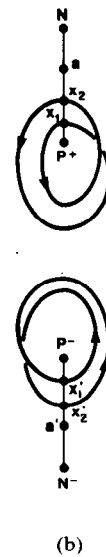
Fig. 23. Two period-2 points X_1 and X_2 with 0 < X_1 < X_2 < a . (a) Graph of 1-D Poincaré map \pi^* . (b) Abstraction of the corresponding periodic orbits in the original double-scroll system.
