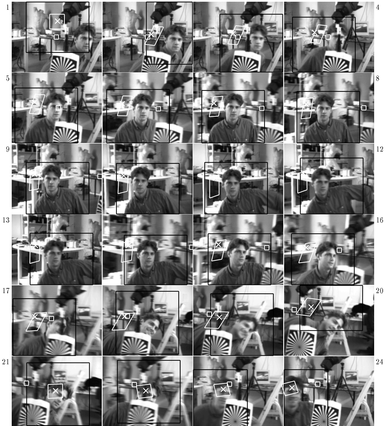
Figure 6: A sequence captured during real-time pursuit. The pursuit system computes an image velocity on every frame (25 per second), to pursue the target. Shown here are every 6 th frame recorded.
