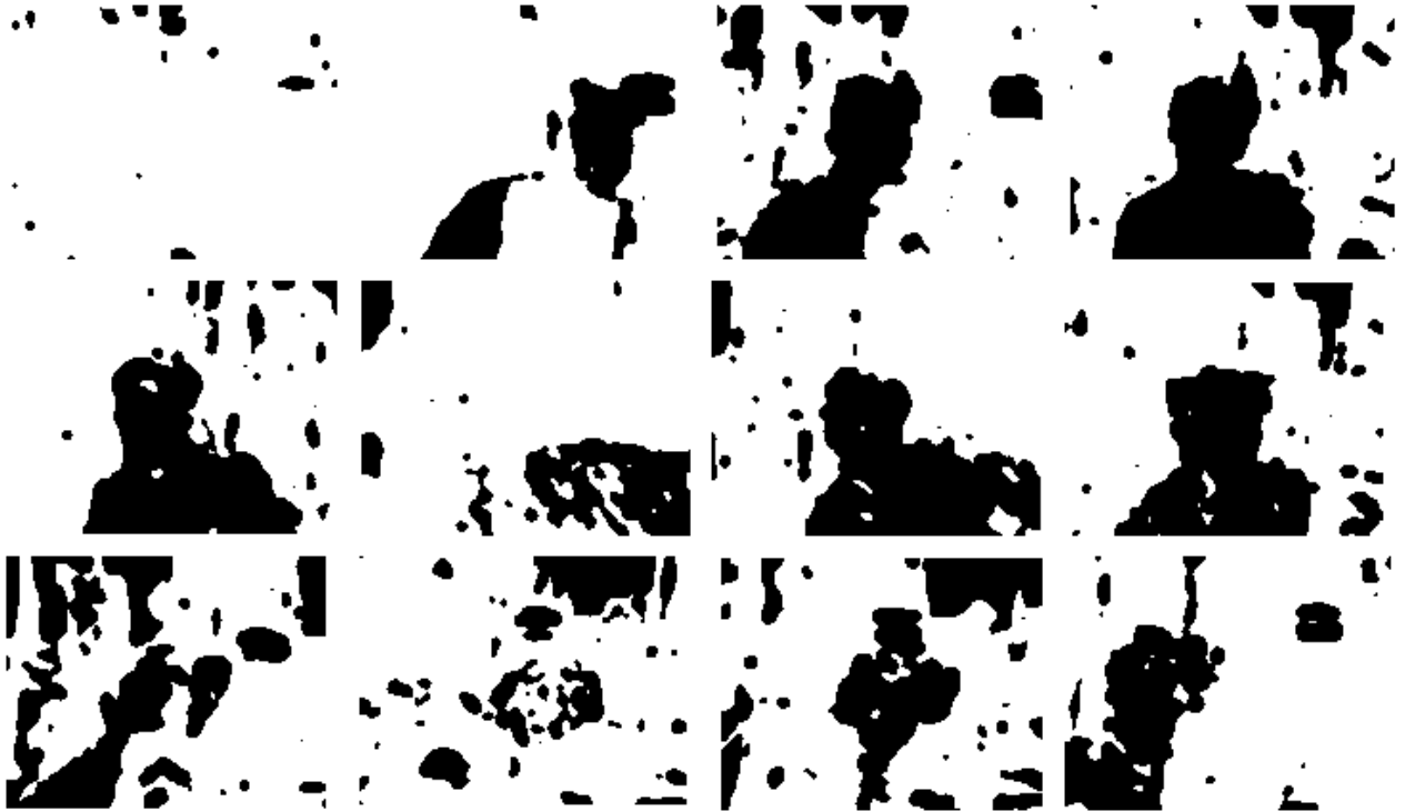
Figure 8: Motion detection returns areas that possibly belong to a moving target. Shown here are the areas which the motion detection marks as possible target pixels. These are the motion detection masks used to produce the final target masks, (compare with odd frames in Figure 7).
