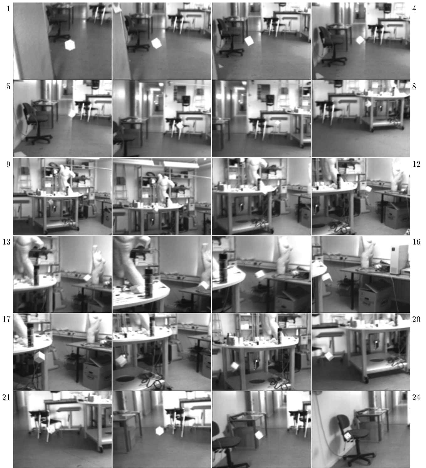
Figure 15: The figure shows the motion detection mechanism with real-time motor-control feedback, tracking the white box. The algorithm is running at 6.5 Hz (for details about the experiment see Section 6.7). The interval is 2 seconds between each frame shown in the figure.
