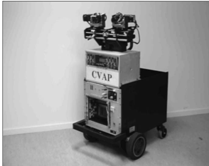
Figure 5: The experimental platform is a Head-Eye-System mounted on a mobile platform.
