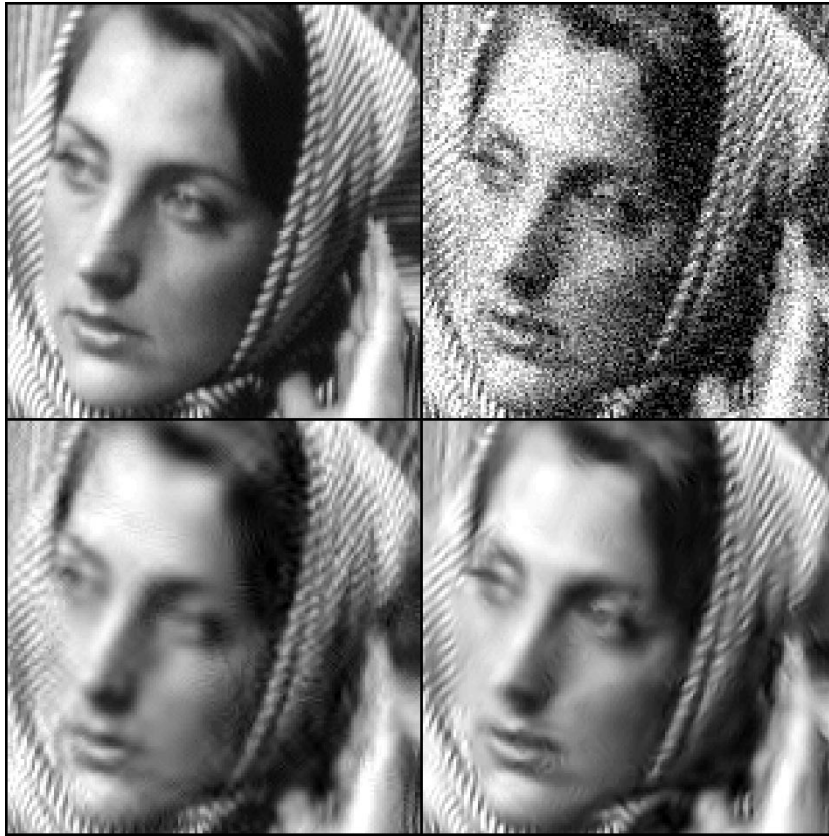
Fig. 6. Comparison of denoising results on Barbara image (cropped to 150 \times 150 for visibility of the artifacts). From left to right and top to bottom: Original image; Noisy image ( \sigma = 25 , PSNR = 20.2 dB); Results of Li et al. [35] ( PSNR = 28.2 dB); Our method ( PSNR = 29.1 dB).
