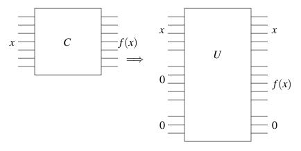
How is this done? Recall that any classical AND and OR gates can be simulated with a C-SWAP gate and some scratch  $|0\rangle$  qubits.
