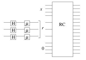
Measurement can be tricky in the intermediate stages of a quantum circuit. Why not skip the measurement and get a superposition of states? Well, if a Hadamard gate occurs in the circuit, we have a problem. The desired outcome is one of these two possibilities with probability 1/2:
