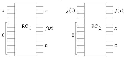
The concatenation  $RC_1$  followed by  $RC_2^{REV}$  is the desired simple circuit.
