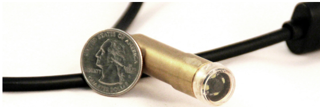
Figure 4. The hardware can be miniaturized, as in this pipe inspection camera with integrated LEDs.
