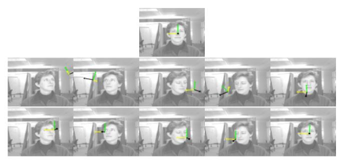
Figure 4. Pose estimation results for real sequence of approx 300 frames (about 10 seconds). Top image: Initial frame in sequence, with result pose axes in initial position. Middle image row: Axes indicate results obtained using BCCE with planar depth for select frames later in sequence. Bottom image row: Results for the same frames using joint BCCE and DCCE with measured depth.
