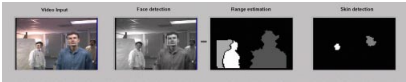
Figure 2. Output of vision processing modules: input image, face pattern detection output, connected components recovered from stereo range data, and flesh hue regions from skin hue classification. Boxes have been drawn on the faces of the two tracked users in the input image; the rightmost person in the image is beyond the workspace of the system.
