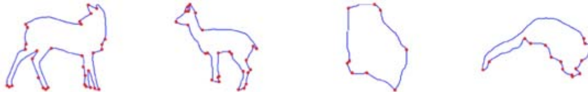
Fig. 2 We take each boundary contour C and break it up at local curvature maxima (corners). Shown are a few examples of this decomposition. The contour segment length |L| is large for large-scale features
