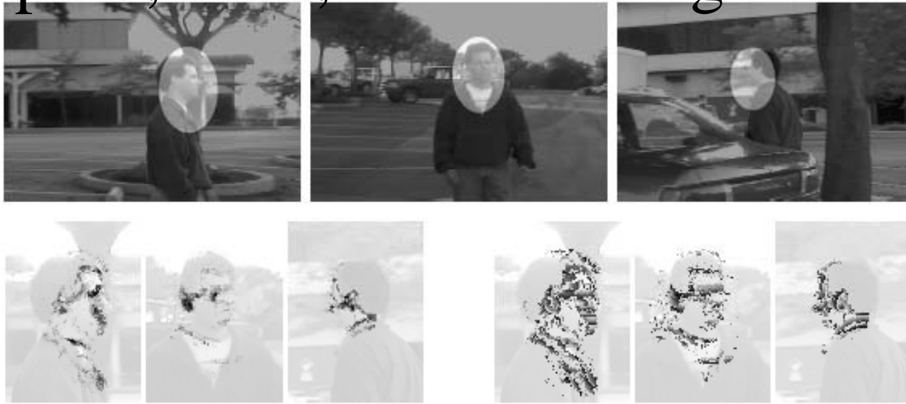
Figure 4. The adaptation of the model during tracking. (top) The target region in selected frames 200, 300, 480. (bottom) The stable component's mixing probability (left) and mean (right) for the selected frames.
