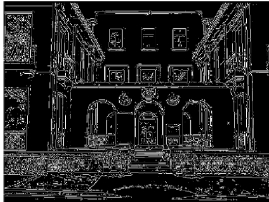
low threshold (weak edges)
