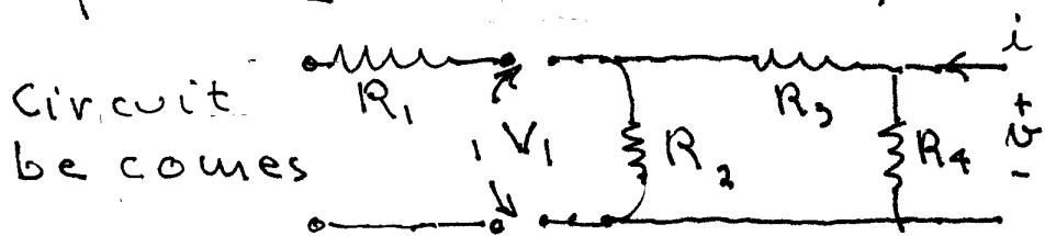
Combine  $R_2$ ,  $R_3$  &  $R_4$  to obtain  $R_{eq}$
