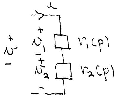
$$\begin{aligned} V &= V_1 + V_2 \\ &= i_1 r_1(p) + i_2 r_2(p) \\ &= i (r_1(p) + r_2(p)) \\ &= i (r(p)) \end{aligned}$$
