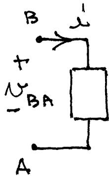
when the current reference is as shown. This implies field puts energy into the element. This can be dissipated or stored
