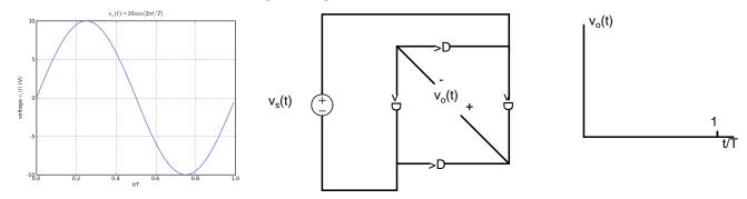
a) for one cycle of a sinusoidal waveform applied  $v_s(t) = 10 \sin(2\pi t/T)$  as shown, sketch the output voltage waveform  $v_o$ .
