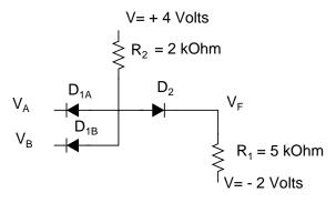
a) Take  $V_A = 5V$ . Use  $V_{D_{on}} = .7V$ . Plot  $V_F$  versus  $V_B$ . b) What type of gate is this for positive logic?
