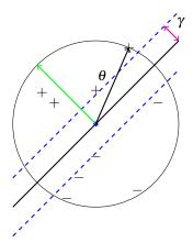
Labelled points with  $x_1, \ldots, x_n$ . Hyperplane separator. Margins. Inside unit ball. Margin  $\gamma$ Hyperplane:  $w \cdot x \geq \gamma$  for + points.  $w \cdot x \leq -\gamma$  for - points. Put points on unit ball.  $W \cdot X = \cos\theta$ Will assume positive labels!
