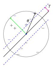
Labelled points with  $x_1, \ldots, x_n$ . Hyperplane separator. Margins. Inside unit ball. Margin  $\gamma$ Hyperplane:  $w \cdot x \ge \gamma$  for + points.  $w \cdot x \leq -\gamma$  for - points. Put points on unit ball.  $W \cdot X = \cos\theta$ Will assume positive labels! negate the negative.
