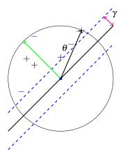
Labelled points with  $x_1, \ldots, x_n$ . Hyperplane separator. Margins. Inside unit ball. Margin  $\gamma$ Hyperplane:  $w \cdot x \ge \gamma$  for + points.  $w \cdot x \leq -\gamma$  for - points. Put points on unit ball.  $W \cdot X = \cos\theta$ Will assume positive labels! negate the negative.
