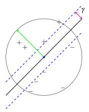
Labelled points with  $x_1, \ldots, x_n$ . Hyperplane separator. Margins. Inside unit ball. Margin  $\gamma$ Hyperplane:  $w \cdot x \ge \gamma$  for + points.  $w \cdot x \le -\gamma$  for - points. Put points on unit ball.
