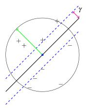
Labelled points with  $x_1, \ldots, x_n$ . Hyperplane separator. Margins. Inside unit ball. Margin  $\gamma$ Hyperplane:
