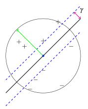
Labelled points with  $x_1, \ldots, x_n$ . Hyperplane separator. Margins. Inside unit ball. Margin  $\gamma$ Hyperplane:  $w \cdot x \ge \gamma$  for + points.  $w \cdot x \le -\gamma$  for - points.
