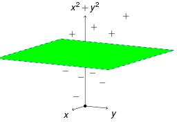
No hyperplane separator. Circle separator! Map points to three dimensions. map point (x, y) to point  $(x, y, x^2 + y^2)$ . Hyperplane separator in three dimensions.
