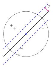
Labelled points with  $x_1, \ldots, x_n$ . Hyperplane separator. Margins. Inside unit ball. Margin  $\gamma$
