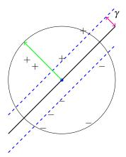
Labelled points with  $x_1, \ldots, x_n$ . Hyperplane separator. Margins. Inside unit ball. Margin  $\gamma$ Hyperplane:  $w \cdot x \ge \gamma$  for + points.
