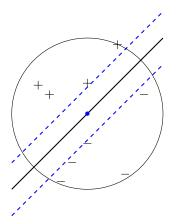
Labelled points with  $x_1, \ldots, x_n$ . Hyperplane separator. Margins. Inside unit ball.
