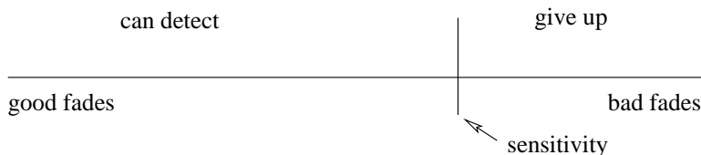
Fig. 28. The probability of missed detection can be conditioned on the depth of the fade encountered. We are going to miss the signal for sure in the bad fades, even if we catch it perfectly when the fading is not so bad.
