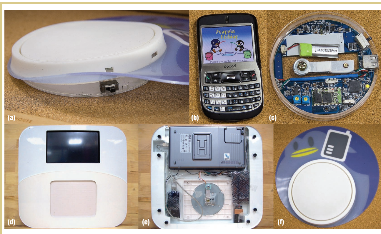
Figure 3. The design of the Playful Tray prototypes: (a) the previous tray prototype; (b) a Palm-top PC and weight sensing surface; (c–d) a placemat sleeve protecting the weight sensing unit; (e) a Bluetooth weight sensing unit that streams weight change events to the mobile phone; and (f) a mobile phone running the Fishing Game.
