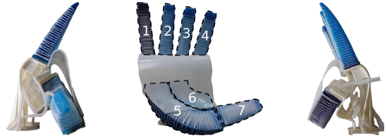
Fig. 2. The RBO Hand 2 is an anthropomorphic pneumatically actuated soft hand consisting of seven actuators. Three of them form the palm and thumb. The air chambers can be physically coupled or actuated separately.
