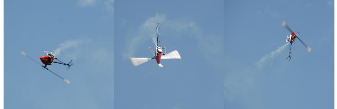
Fig. 1. The dynamical modeling method presented in this work is used to model a helicopter’s dynamics as it is flown through aerobatics. A unified model is learned for a rich array of maneuvers, including flips, loops, stop and go, vertical sweeps, circles, dodging, orientation sweeps, gentle freestyle, tictocs, chaos, and aggressive freestyle.
