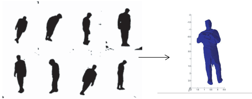
Figure 3-1: At each frame i , silhouette images produce a polyhedral triangle mesh.
