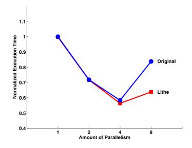
Figure 7-10: Performance comparison of the original and ported implementation of the FFTW library computing an FFT of size 131,072.
