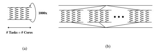
Figure 7-1: (a) The baseline barrier microbenchmark of N SPMD tasks synchronizing with each other 1000 times at back-to-back barrier rendezvous. (b) Launching multiple baseline barrier microbenchmarks in parallel to examine the behavior of different barrier implementations in the face of parallel composition.
