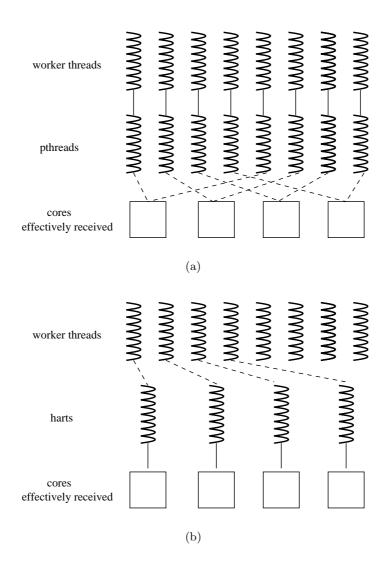
Figure 6-4: (a) The original OpenMP implementation maps each worker thread to a pthread, effectively leaving all scheduling decisions to the OS. (b) The Lithe OpenMP implementation maps each worker thread to a hart in a more efficient manner, executing each worker thread to completion to eliminate unnecessary context switching and interference.
