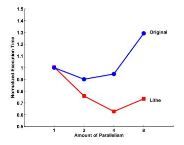
Figure 7-11: Performance comparison of the original and ported FFTW implementation of the FFTW library computing an FFT of size 32,768.
