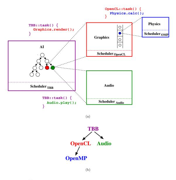
Figure 2-1: (a) The hierarchical call structure of the example gaming application. The AI component invokes the graphics and audio components as two of its TBB tasks. The graphics component, in turn, invokes the physics component as one of its OpenCL tasks. (b) The corresponding hierarchy of schedulers. TBB allocates resources between OpenCL, the custom audio scheduler, and itself. OpenCL allocates resources between OpenMP and itself.
