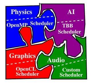
Figure 1-3: An example gaming application composed of several parallel components, which are built in turn using different parallel libraries. The physics component is written using OpenMP [CMD<sup>+</sup>01]. The AI component is written using TBB [Rei07], the graphics component is written using OpenCL [Gro]. The audio component is written using a customized framework.
