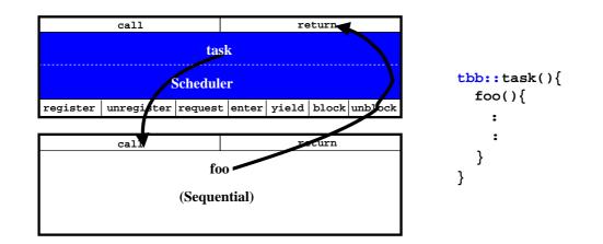
Figure 4-1: The Lithe scheduler callback interface, which is orthogonal to the function call interface, enables the plug and play of an OpenMP, Cilk, or sequential implementation of foo. Furthermore, there is a separation of concerns between the high-level functionality of task invoking foo, and the low-level resource management of their respective schedulers exchanging harts.
