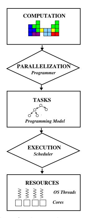
Figure 1-2: The two main steps of mapping computation onto resources, encapsulated within each parallel software component. First, the programmer decomposes the computation into tasks. Then, the scheduler executes the tasks with its resources. The parallel programming model provides the task abstraction, and governs how computation behaviors and needs are translated into execution policies.
