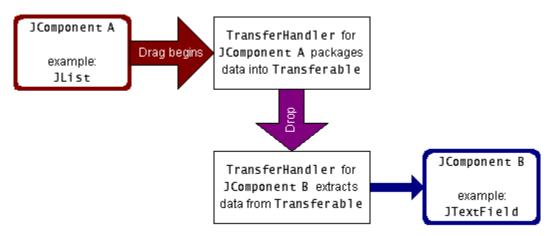
Figure 5-4: The Use of Swing Transfer Handlers in Drag and Drop
