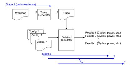
Figure 2-1. Trace-driven simulation
