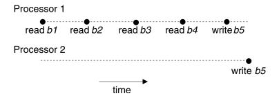
Figure 3-4. Scenario illustrating why write accesses are recorded in the MTR as read-modify-write. Assume a four-way associative cache with LRU replacement. Blocks b1-b5 map to the same set. We need to retain the time of P1's write to b5 to reconstruct the eviction of b1.
