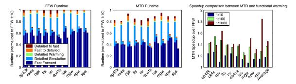
Figure 3-17. Normalized running time of FFW and MTR and the relative speedup of MTR over FFW. Each group of three bars represents the run time with detailed-to-fast ratios of 1:10, 1:100, and 1:1000. Each bar separately shows time spent in the three phases of simulation including transitions.
