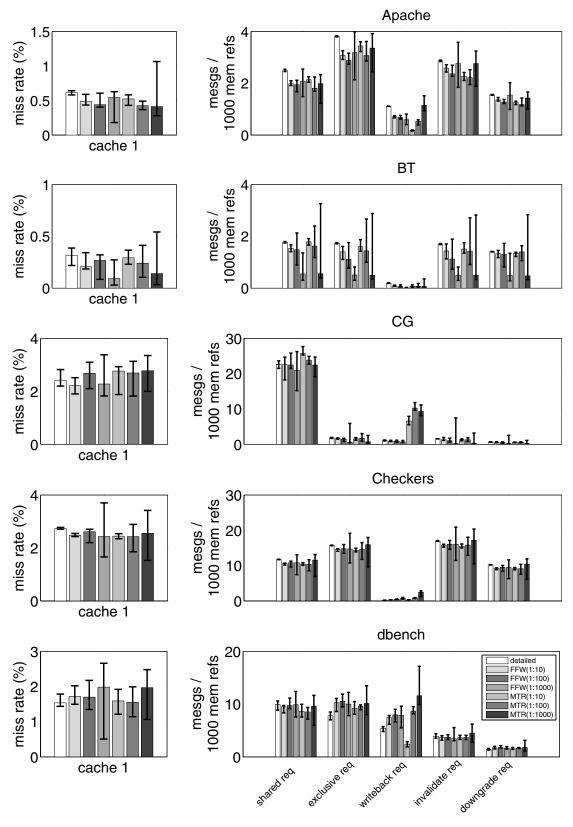
Figure 3-15. Accuracy comparison of FFW and MTR to detailed simulation. Each bar represents the median of eight individual runs of the benchmark. Max and min are noted with thin lines. No ambiguity resolution is performed.
