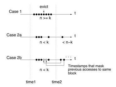
Figure 3-11. Different scenarios when reconstructing evictions. The MTR contains entries marked time1 and time2. The black dots represent accesses recorded in the MTR; the white dots represent accesses no longer visible in the MTR. In the first case, we know for sure that the eviction occurred before the memory access, whereas the second case is ambiguous because of the possibly missing timestamps from the MTR.
