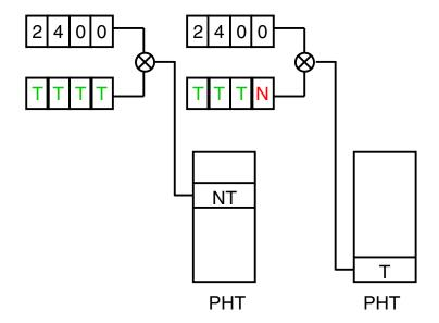
Figure 4-3. Anti-aliasing maps a single branch to multiple PHT entries depending on context.
