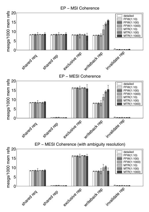
Figure 3-16. Comparison of MSI and MESI protocols. The bottom figure shows the reduction in writeback messages caused by resolving M/S ambiguities as described in Section 3.1.5.
