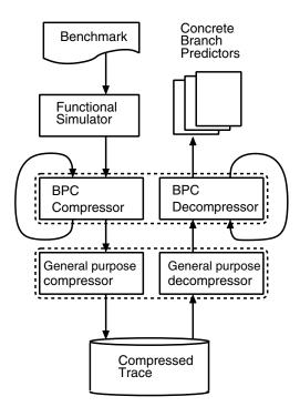
Figure 4-4. System diagram. The compressed trace is stored on disk until it is needed to reconstruct concrete branch predictors.
