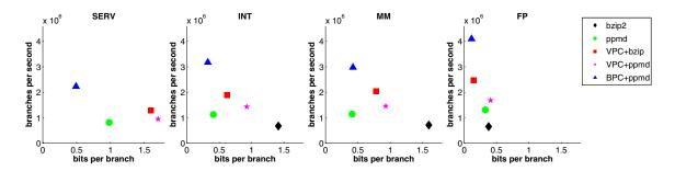
Figure 4-10. Decompression speed vs. Compressed Ratio. The optimal compressed trace format is in the upper left of each plot. Decompression speed across applications is reported with harmonic mean.
