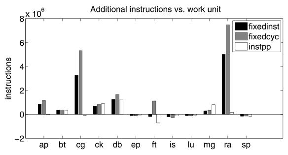
Figure 5-1. Additional execution resulting from incorrect sample bounds.
