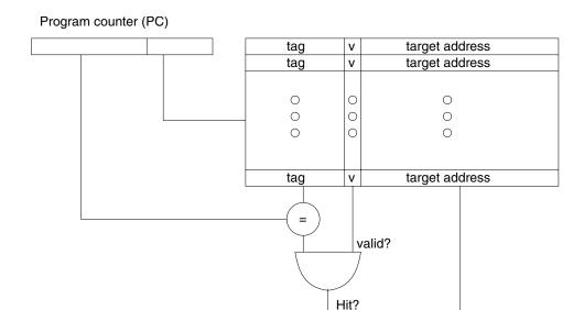
Figure 4-1. A branch target buffer (BTB). A canonical BTB is updated only with taken branches. Thus, hits in the BTB indicate the lookup PC is a taken branch.
