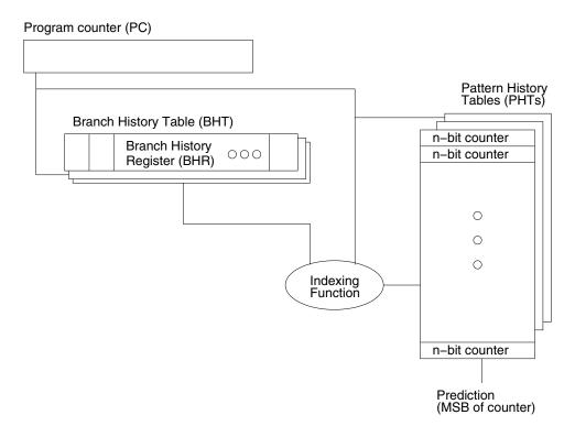
Figure 4-2. Parts of a canonical two-level adaptive branch predictor.
