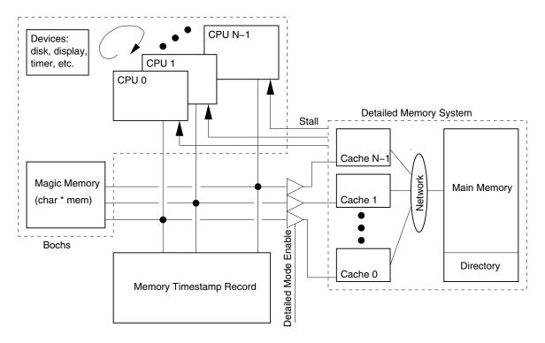
Figure 3-13. Evaluation infrastructure. The detailed memory model stalls a processor's execution based on timing models.
