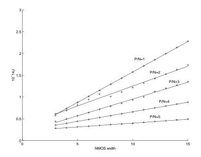
Figure 3-15: Measurements of fall short-circuit energy for various inverters.
