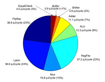
Figure 5-1: Average energy breakdown by component type.
