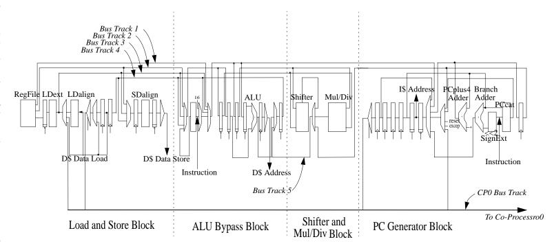
Figure 4-4: Floorplan of datapath (except coprocessor 0).
