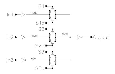
Figure 3-1: A 3-input Transmission-gate mux.
