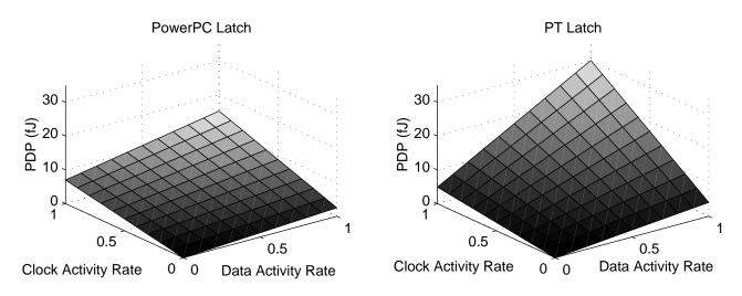
Figure 2-12: PDP of latches.
