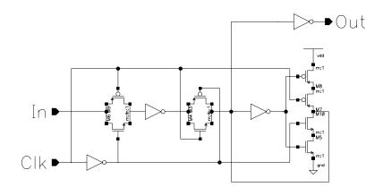
Figure 2-2: Modified PowerPC flipflop.
