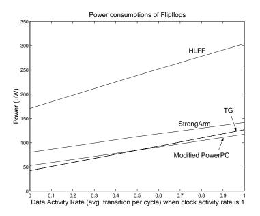
Figure 2-6: Power dissipation of flipflops (clock activity=1).
