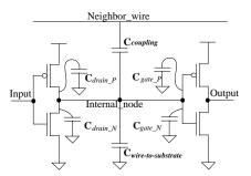
Figure 3-5: Schematic of cascaded inverters and the capacitances connected to the internal\_node.
