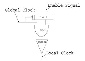
Figure 4-16: Clock gating circuit.
