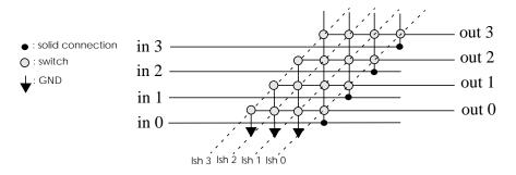
Figure 4-7: A barrel shifter.
