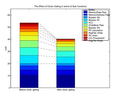
Figure 5-10: The effect of clock gating in terms of sub-functional blocks.
