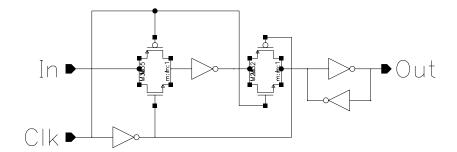
Figure 2-5: Transmission-gate flipflop.
