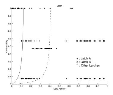
Figure 5-7: Clock and data activities for various latches. A solid curve is a PDP curve and a dashed curve is a power curve.
