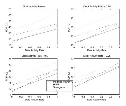
Figure 2-9: PDP of flipflops when clock activity rate is fixed.
