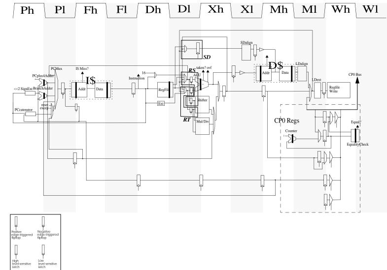
Figure 4-1: Pipeline diagram for datapath.
