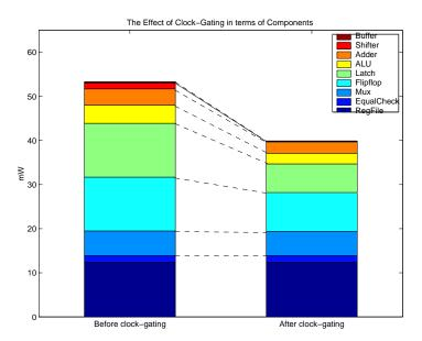
Figure 5-8: The effect of clock gating in terms of components.
