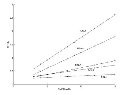
Figure 3-16: Measurements of rise short-circuit energy for various inverters.
