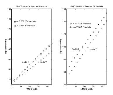
Figure 3-10: Deriving gp, dp, gn and dn from measurements.
