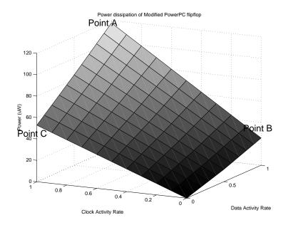
Figure 2-7: Power dissipation of modified PowerPC flipflop.
