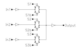
Figure 2-14: Transmission-gate mux.
