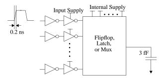
Figure 2-1: Test bench for flipflops, latches, and muxes.
