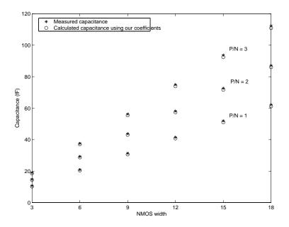
Figure 3-11: Verification of gate and drain capacitance coefficients. P/N is the ratio of PMOS width to NMOS width.
