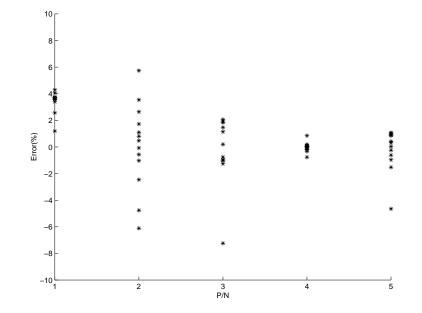
Figure 3-17: Error between the measured average short-circuit energy and the calculated one using table lookup.
