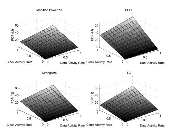
Figure 2-8: PDP graphs of flipflops.
