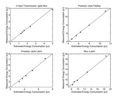
Figure 3-13: Mux, latch, flipflop and mux-latch: measured energy vs. estimated energy. Ideally, all points should fall on the line.
