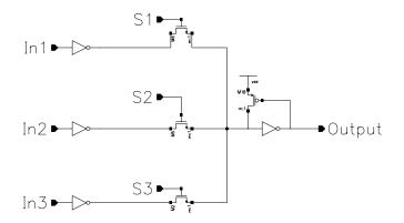
Figure 2-15: Pass-transistor mux.
