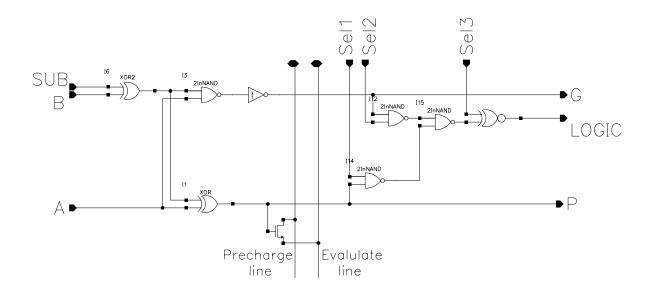
Figure 4-6: Modified propagate(P) and generate(G) circuit for ALU.
