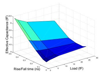
Figure 3-4: Sum of an inverter's PMOS and NMOS drain capacitances.
