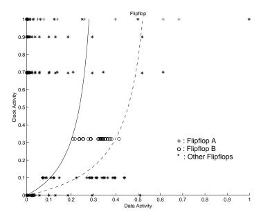
Figure 5-6: Clock and data activities for various flipflops. A solid curve is a PDP curve and a dashed curve is a power curve.
