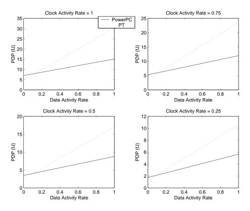
Figure 2-13: PDP of latches when clock activity is fixed.
