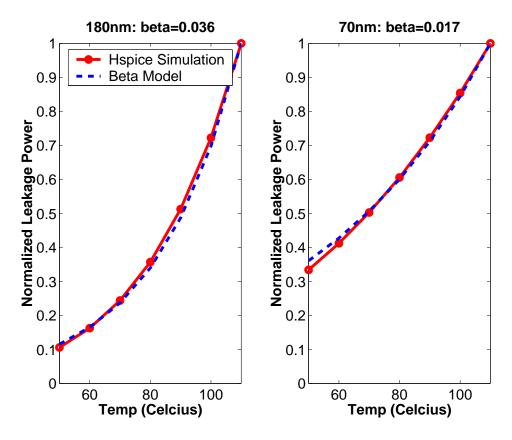
Figure 8-2: Leakage power versus temperature.
