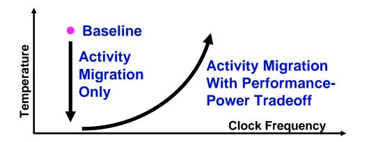
Figure 8-5: Conceptual benefits of AM: reduced temperature or increased frequency due to possibility to perform dynamic voltage scaling.
