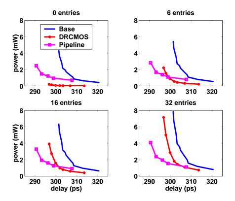
Figure 5-35: PD curves for arbiter using transistor sizing.
