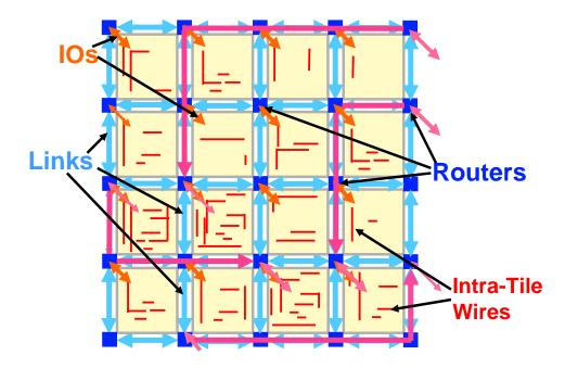
Figure 7-8: Tiled packet-routed ASIC design.
