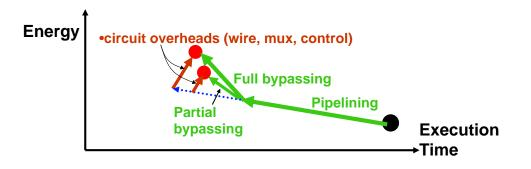
Figure 4-4: Bypassing to overcome data dependences.
