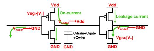
Figure 3-2: Decomposing a digital circuit: currents and parasitic capacitances of transistors and voltages.  $C_{drain}$ ,  $C_{gate}$ , and  $C_{wire}$  are the parasitic transistor drain and gate caps, and wire cap respectively.
