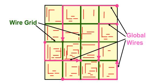
Figure 7-5: Wire-routed ASIC design.
