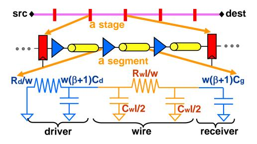
Figure 7-2: First-order RC model of wire. The length of the whole wire is L.  $\beta$  is the PN ratio, w is the width of the repeater NMOS transistor,  $C_w$ ,  $C_d$ , and  $C_g$  are the unit-length wire cap and drain and gate caps of the minimum-sized inverters respectively.
