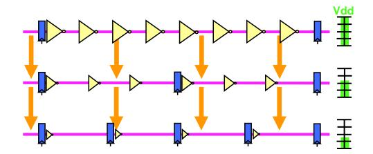
Figure 7-1: Pipelining wires and scaling supply voltages for energy reduction at a fixed bandwidth.
