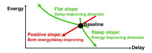
Figure 2-1: Energy-delay tradeoffs with different slopes.
