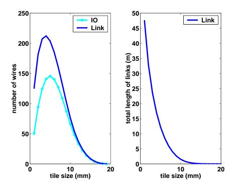
Figure 7-9: Number and total length of inter-tile wires.
