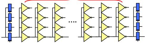
Figure 6-2: Baseline pipeline stage model. Input and clock buffers are not shown.
