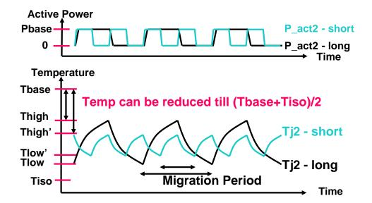
Figure 8-6: Analytical calculation of benefits of AM.  $T_{base}$  is the baseline temperature,  $T_{iso}$  is the isothermal point,  $T_{high}$  and  $T_{low}$  are the highest and lowest temperatures for AM technique, and *Period* is AM period.
