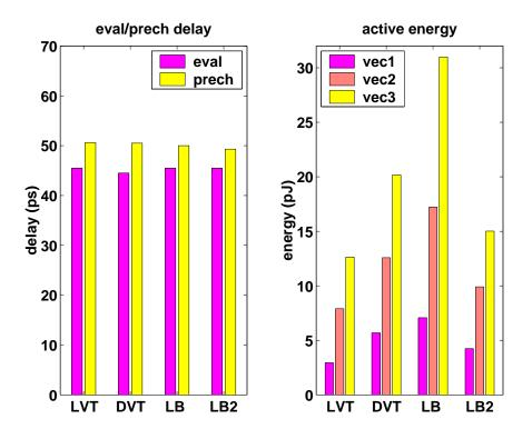
Figure 5-20: Delay and switching energy consumption : 70 nm process.
