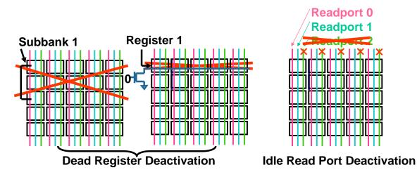
Figure 5-11: Dead register deactivation and idle port deactivation for register files.
