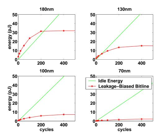
Figure 5-8: Idle energy and LBB energy of 32-row×16B SRAM subbank for different processes (optimistic leakage current was used).
