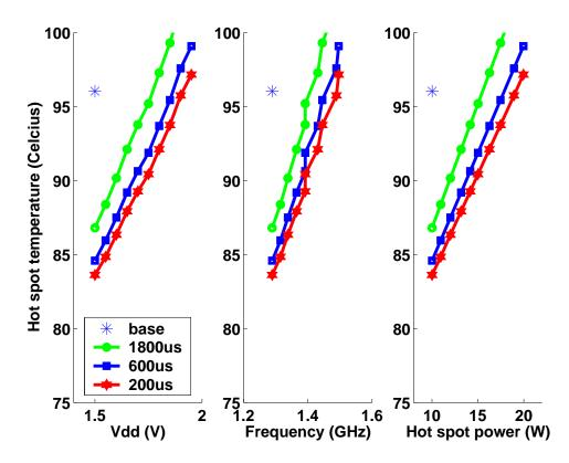
Figure 8-8: Simulation results of AM and DVS for various AM periods (Current case)
