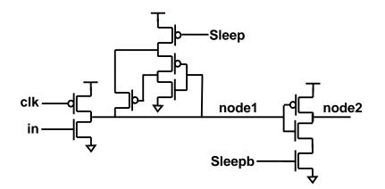
Figure 5-17: A leakage-biased domino buffer.
