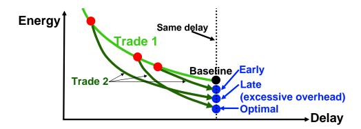
Figure 2-5: Optimal combination of energy-delay tradeoffs for maximum energy saving.
