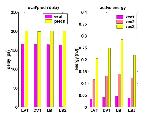
Figure 5-19: Delay and switching energy consumption : 180 nm process.
