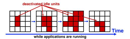
Figure 4-16: Temporally and spatially fi ne-grain dynamic deactivation.
