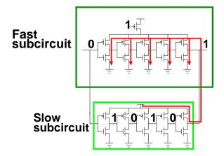
Figure 5-28: Sneak leakage path problem.
