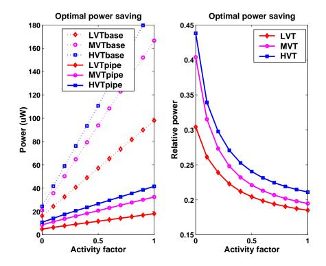
Figure 6-10: Optimal power saving with no clock-gating mechanism.
