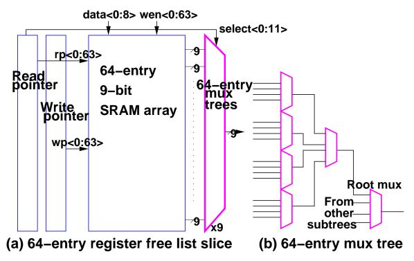
Figure 5-29: A static 64-entry register free list slice.
