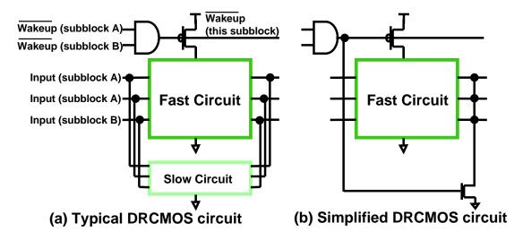
Figure 5-27: Dynamically resizable static CMOS logic (DRCMOS).
