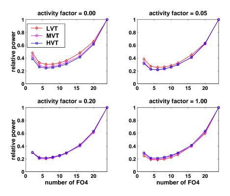
Figure 6-7: Total power scaling with a clock-gating mechanism.
