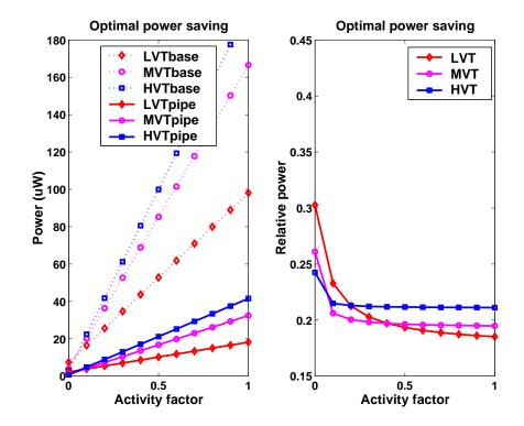
Figure 6-8: Optimal power saving with a clock-gating mechanism.
