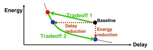
Figure 2-4: Combining energy-delay tradeoffs for delay reduction at the same energy or energy saving at the same delay.
