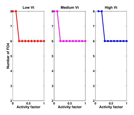
Figure 6-11: Optimal logic depth with no clock-gating mechanism.
