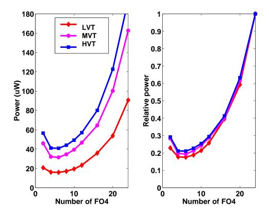
Figure 6-4: Switching power scaling.
