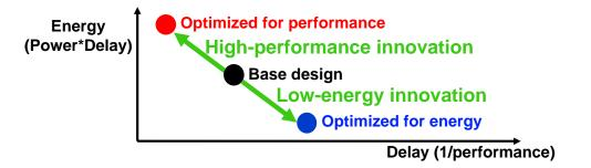
Figure 1-2: Energy-delay tradeoffs: optimizing for either greater performance or lower energy.
