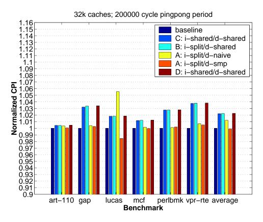
Figure 8-12: CPI with 32KB Caches (2 Cycles Hit Latency)
