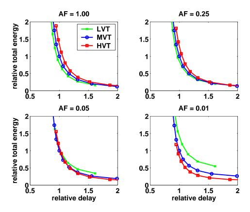
Figure 3-11: Scaling supply voltage for different threshold voltages and activity factors. AF is the activity factor and LVT, MVT, and HVT are low-threshold, medium-threshold, and high-threshold transistors respectively. Switching energy, leakage power, and delay are normalized to the MVT and nominal  $V_{dd}$  point.
