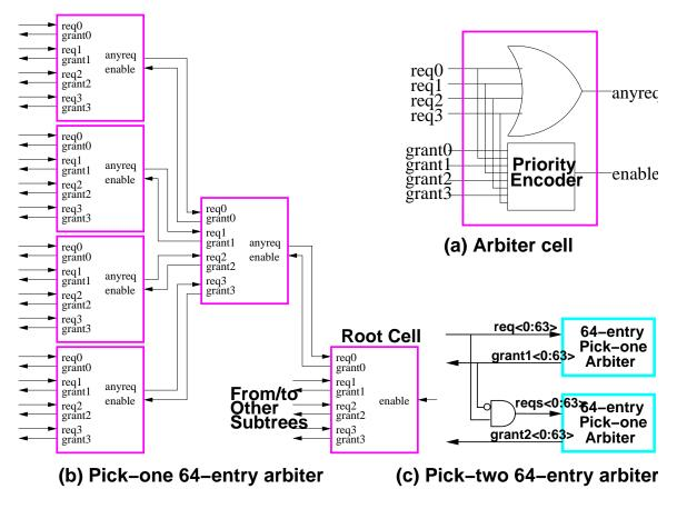
Figure 5-30: A static 64-entry pick-two arbiter.
