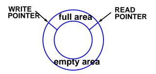
Figure 5-31: Logical structure of issue window.
