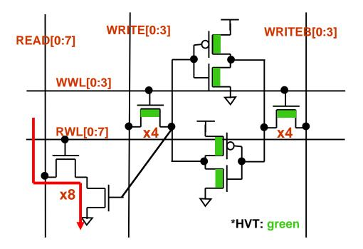
Figure 5-9: An embedded dual  $V_T$  unbalanced 8-read, 4-write register fi le cell.
