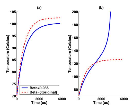
Figure 8-3: Comparison of thermal models. Simulation is based on Current case and we assume that  $T_j$  starts from T. Different switching and leakage power conditions are assumed for simulation (a) and (b).
