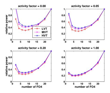
Figure 6-9: Total power scaling with no clock-gating mechanism.
