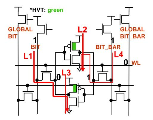
Figure 5-5: A dual- $V_T$  SRAM cell.
