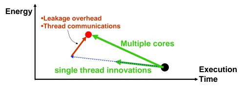
Figure 4-9: Utilizing multiple cores.
