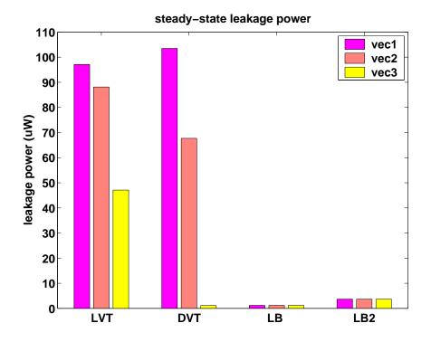
Figure 5-21: Steady-state leakage power : 180 nm process. clk is high for all and sleep is asserted for LB and LB2.
