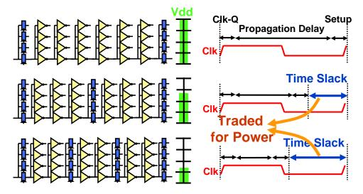
Figure 6-1: Pipelining datapath for lower energy.
