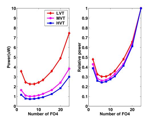
Figure 6-5: Leakage power versus logic depth per stage.
