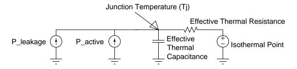
Figure 8-1: Thermal model: an equivalent RC circuit.
