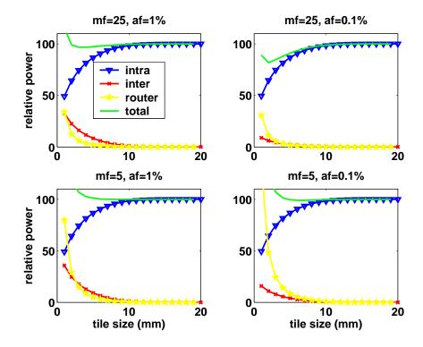
Figure 7-12: Packet-routed ASIC with real routers: power consumption.
