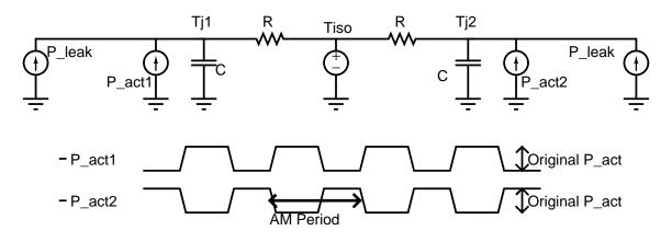
Figure 8-4: AM thermal model : an equivalent RC circuit.
