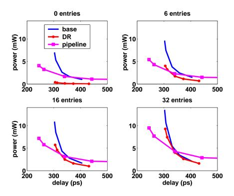
Figure 5-34: PD curves for arbiter using supply voltage scaling.
