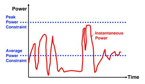
Figure 2-6: Two power constraints for digital systems.
