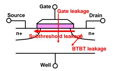
Figure 2-7: Leakage components of deep submicron transistors.
