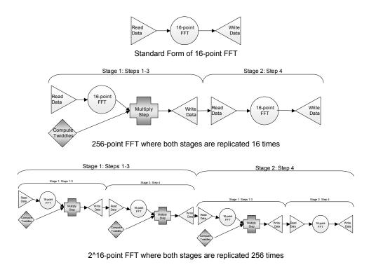
Figure 3-8: Diagram Illustrating Iterative 4-Step Approach
