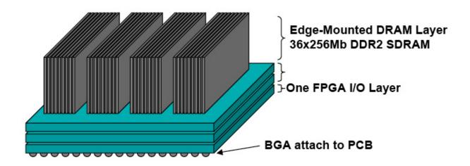
Figure 1-1: Overall 3D FPGA Diagram
