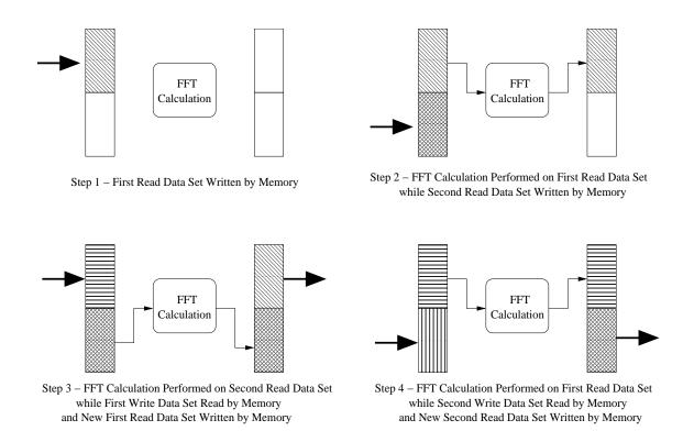
Figure 2-4: FFT Calculation and Memory Flow Diagram
