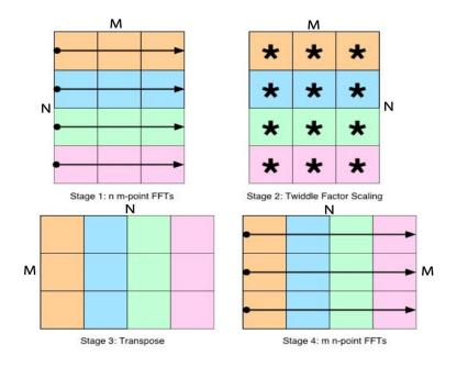
Figure 2-5: 4-Step FFT Method
