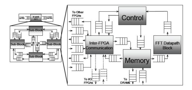
Figure 3-6: UTL Single FPGA System Block Diagram
