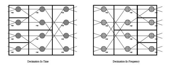
Figure 2-2: DIT Compared to DIF Diagram
