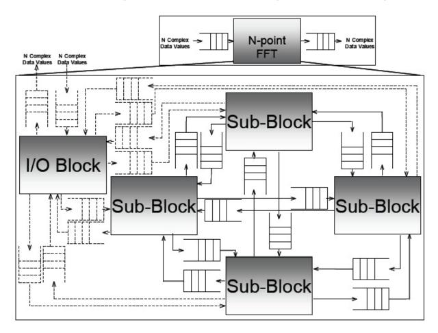
Figure 3-2: Four FPGA UTL Block Diagram
