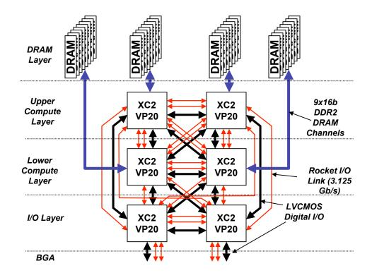
Figure 3-5: Overall Block-Level 3D FPGA System Diagram
