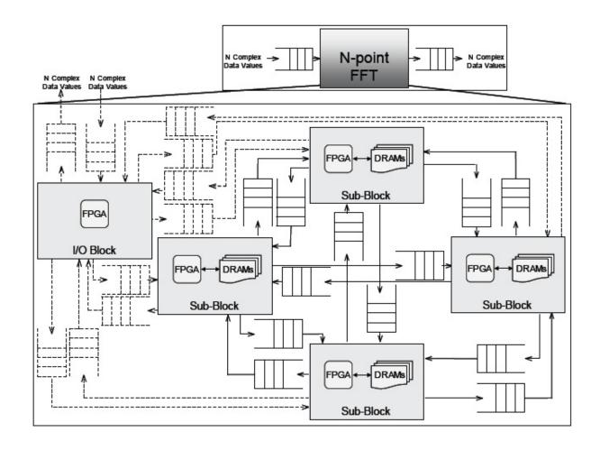
Figure 3-4: Four FPGA Micro-Architectural Block Diagram
