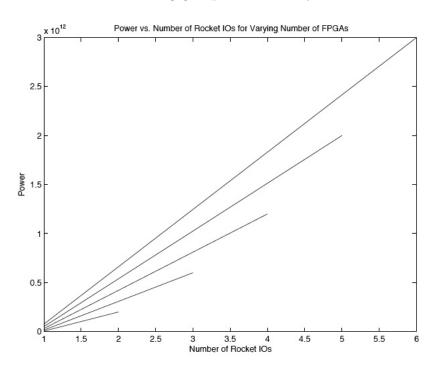
Figure 5-1: Graph Showing the Linear Power Relationship for 2-6 FGPAs
