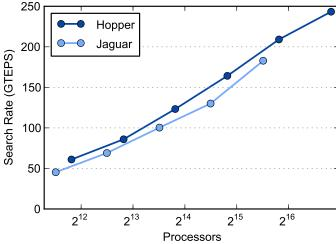
Fig. 3. R-MAT weak scaling comparison between Jaguar and Hopper. Jaguar starts with 2916 processors and Hopper starts with 3600 processors for scale=30 and the number of processors doubles for each increase in scale.
