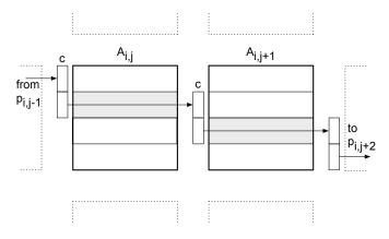
Fig. 1. Sub-step for processors  $p_{i,j}$  and  $p_{i,j+1}$ . They initially use their segment of completed (c) to filter which vertices to process from the shaded region and update completed for each discovery. At the end of the substep, the completed segments rotate to the right. The parent updates are also transmitted at the end of the sub-step (not shown).
