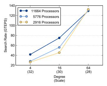
Fig. 7. R-MAT graph with 16B edges with direction-optimizing BFS on Jaguar. Degree varied by changing number of vertices (scale).
