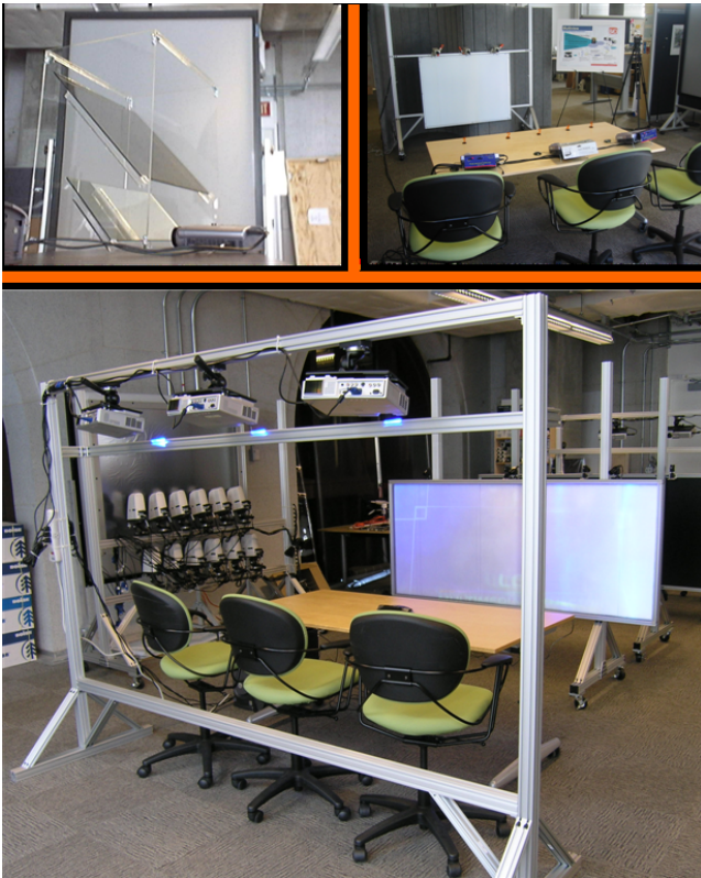
Figure 4. This figure shows the several iterations of MultiView's design. MultiView started as a video tunnel setup with a retroreflective screen (upper left). The video tunnel was abandoned for a front projected directional screen (upper right). The latest iteration includes a larger screen, higher precision optics, short throw projectors, and high resolutions cameras.
