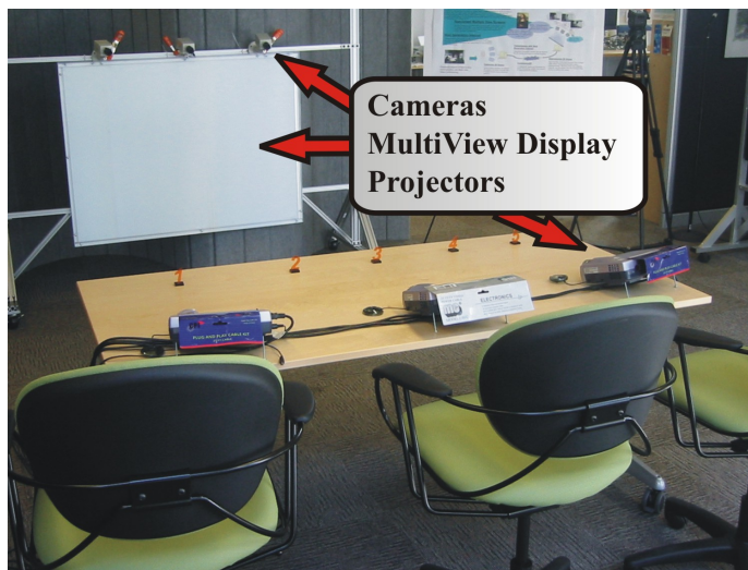
Figure 1: This photograph shows a MultiView site which supports up to three participants and can provide three perspectives. Notice MultiView consists of multiple cameras, multiple projectors, and a specially designed screen. Two setups like this were used in our evaluation.
