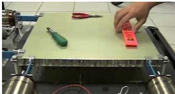
Figure 6.1: The Universal Planar Manipulator (UPM): generic objects placed on a flat plate can be manipulated independently via vibrations/friction.
