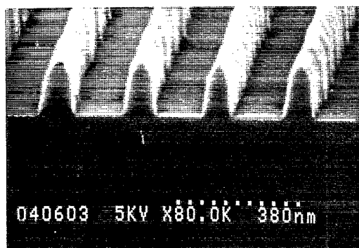
FIG. 2. Electron microscope picture of a silicon grating target, with period 2400 \text{ \AA} and groove depth \approx 1700 \text{ \AA} .
