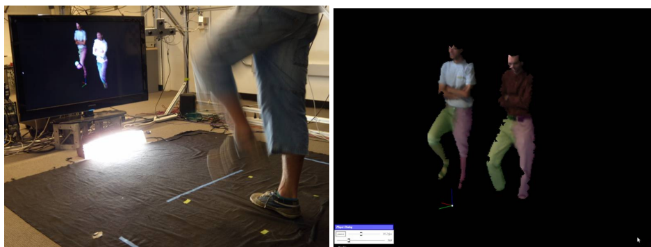
Figure 2. Stereo reconstruction is used to capture user's 3D avatar in real time (left) and project it into a shared virtual environment (right), enabling a patient and therapist to interact remotely. Color shading of the legs assists with focus and orientation within the virtual mirror projection.
