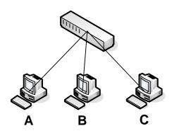
Topology used for better performance. When A sends a lot, B is not prevented from sending – unlike the shared Ethernet, when packets from A and B would cause congestion on the shared medium.
