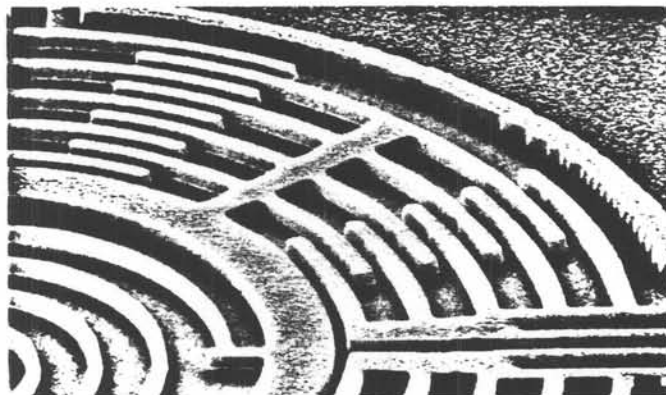
Fig. 8. SEM micrograph of the concentric comb structure.
