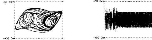
(a) VC2 as function of VC1 (b) VC2 as function of time Fig.6, external amplitude F=200mV
