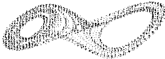
Fig. 3 The attractor projected on a V_{c1} - V_{c2} plane ( R = 1.334 \text{ k}\Omega ). This attractor is double scroll attractor which is a typical one in the Chua's circuit ( R = 1.334 \text{ k}\Omega ). This attractor is constructed through the connection of two screw attractors.
