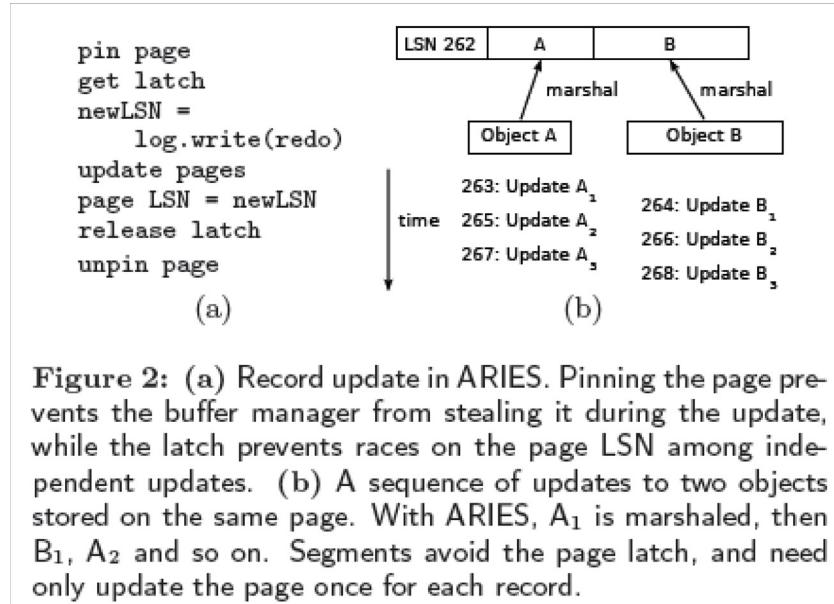
**Figure 2:** (a) Record update in ARIES. Pinning the page prevents the buffer manager from stealing it during the update, while the latch prevents races on the page LSN among independent updates. (b) A sequence of updates to two objects stored on the same page. With ARIES, A<sub>1</sub> is marshaled, then B<sub>1</sub>, A<sub>2</sub> and so on. Segments avoid the page latch, and need only update the page once for each record.
