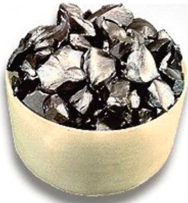
Raw material — Polysilicon nuggets purified from sand
