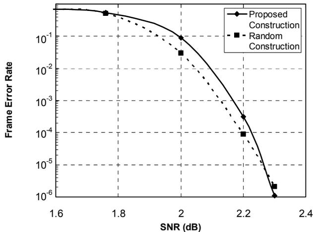
Figure 2. BER curves for proposed LDPC codes, maximum 64 iterations.
