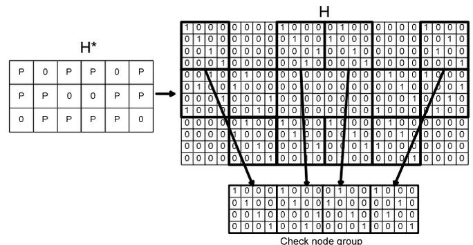
Figure 3. Formation of parity check matrix,  $\mathbf{H}$ , from top level matrix  $\mathbf{H}^*$  and matrix for one check node group.
