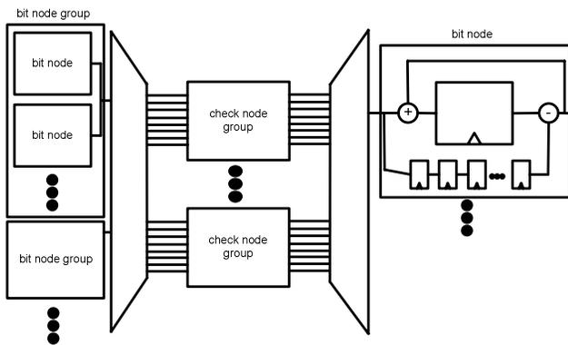
Figure 5. Second implementation of partially parallel decoder.
