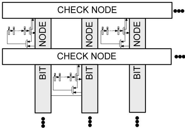
Figure 4. Shift-register structure for LDPC decoders.
