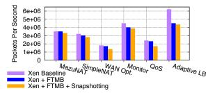
Figure 10: Impact of FTMB on forwarding plane throughput.
