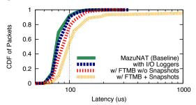
Figure 5: Local RTT with and without components of FTMB enabled.
