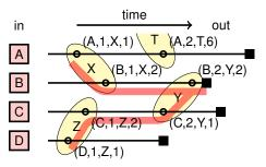
Figure 3: Four threads (black lines) process packets A, B, C, D. As time goes (left to right), they access (circles) shared variables X, Y, Z, T generating the PALs in parentheses. The red tree indicates the dependencies for packet B.
