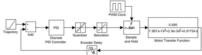
Fig. 12: Simulink model of the motor and PID controller.
