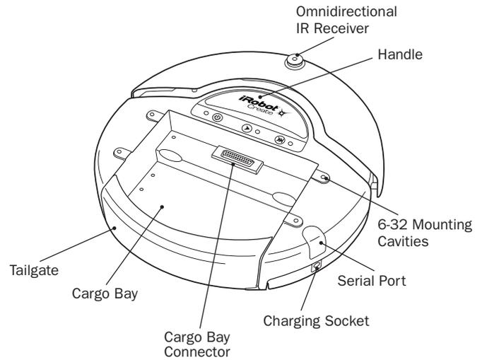
Fig. 1: iRobot Create [27] robotics platform. Source: iRobot Corporation.
