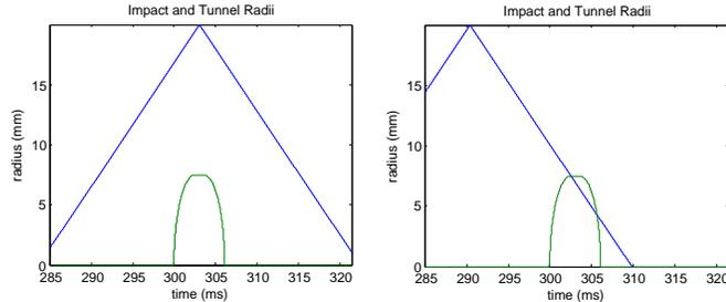
(a) Ball passes through the center of the door. The impact radius is always smaller than the tunnel radius, resulting in success. (b) Ball does not pass through the center of the door. The impact radius becomes larger than the tunnel radius at  $t \approx 302$ ms, resulting in failure.
