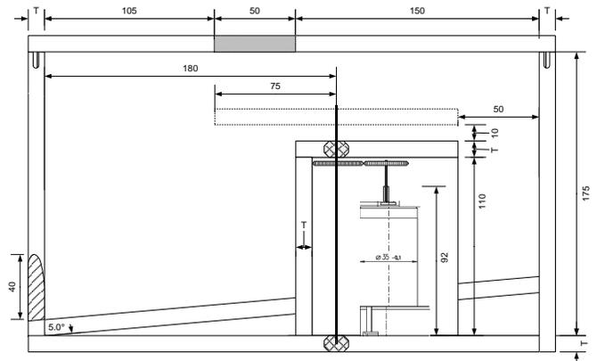
Fig. 23: Tunneling Ball Device drop basin side view.
