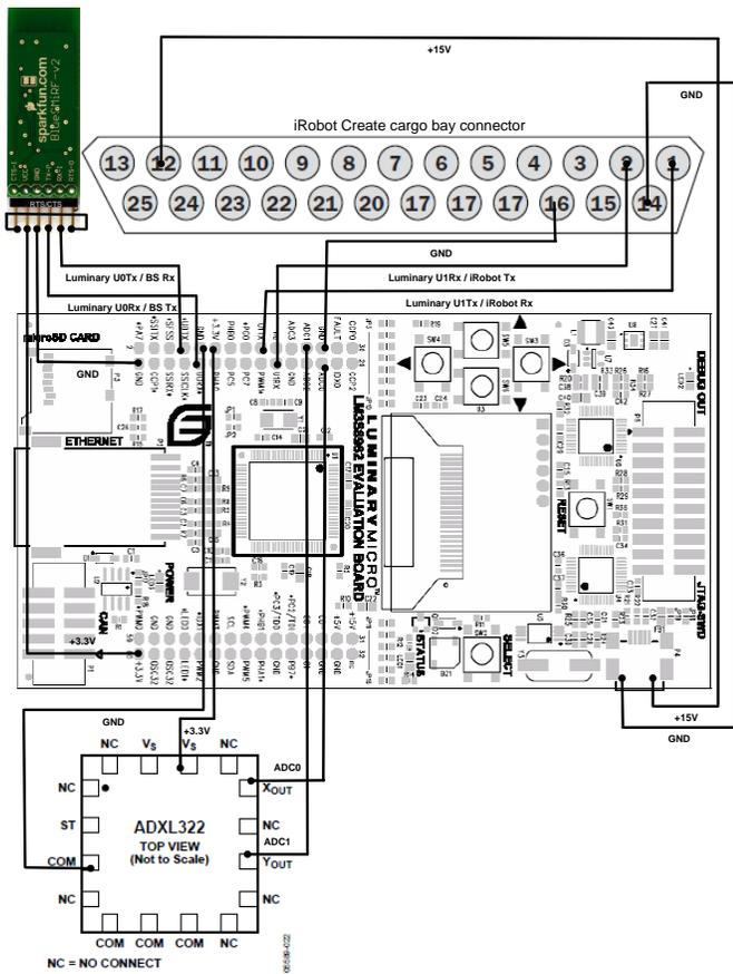
Fig. 21: Wiring diagram for the Cal Climber
