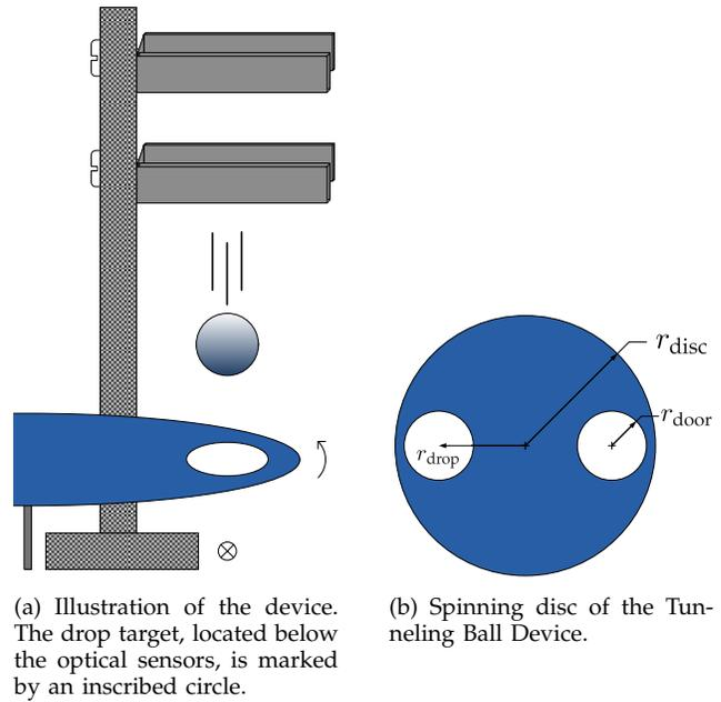
Fig. 6: The Tunneling Ball Device
