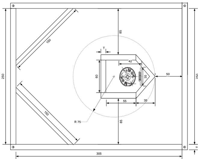
Fig. 22: Tunneling Ball Device drop basin top view.
