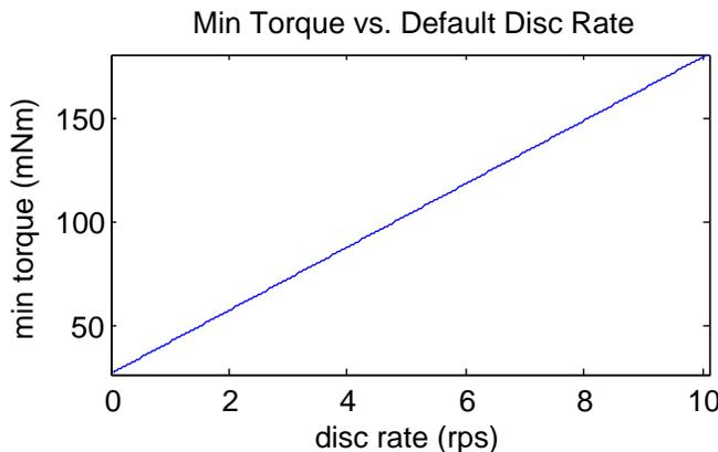
Fig. 15: Minimum torque necessary for  $\mathbf{S}$  for varied  $\omega_0$ . Motor constants were substituted from the datasheet for a Maxon Re-35 motor [33].
