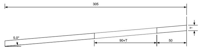
Fig. 24: Tunneling Ball Device floorboard side view.
