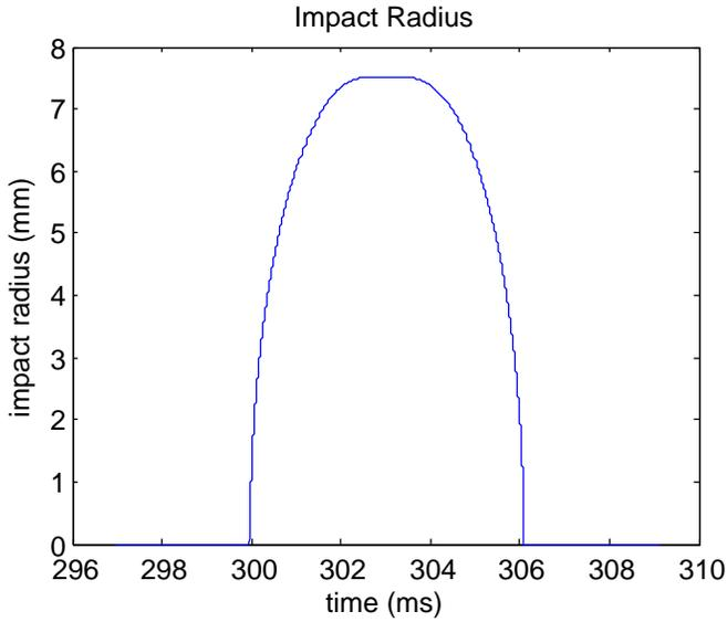
Fig. 7: Impact radius of a 7.5mm radius ball dropped from a height of 400mm. The impact radius is equal to the radius of the ball while the center of the ball passes through the thickness of the disc.
