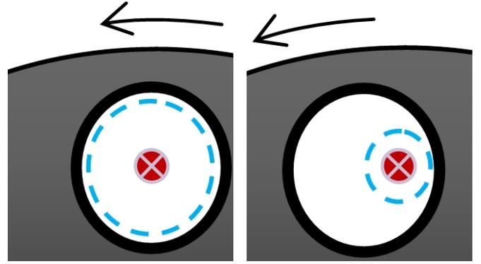
(a) Disc rotated with the door centered over the drop target (optimal tunnel). (b) Disc rotated with the door offset from the drop target (sub-optimal tunnel).
