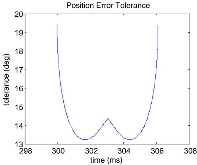
Fig. 10: Simulated position tolerance. The tolerance is always nonzero, indicating the ball does not impact the disc.
