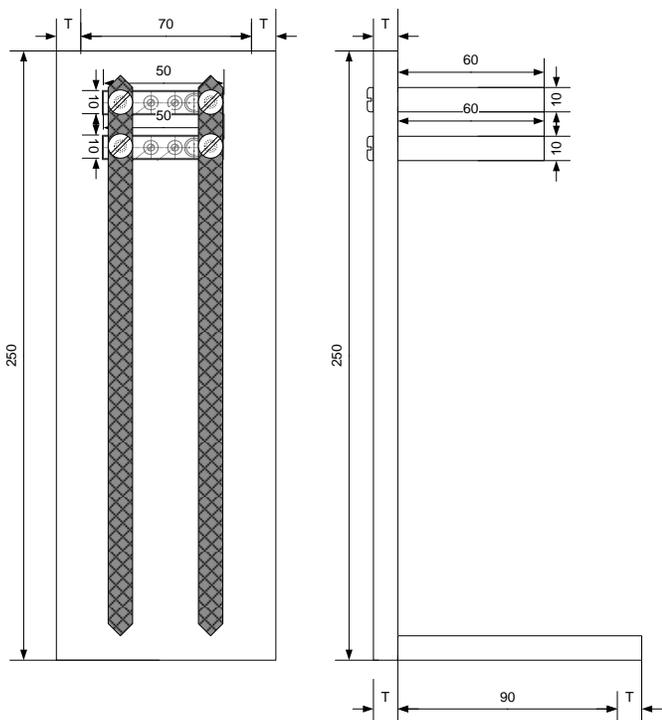
Fig. 26: Tunneling Ball Device drop sensor side view.
