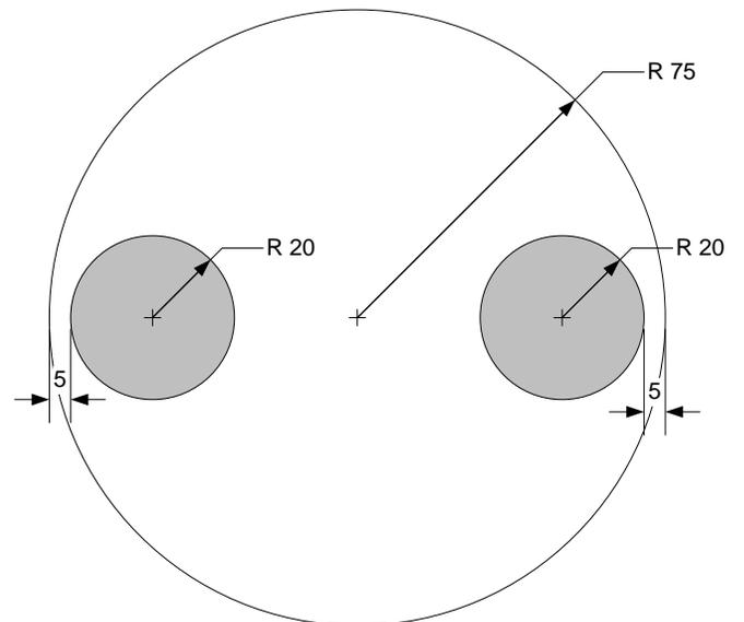
Fig. 28: Tunneling Ball Device disc.
