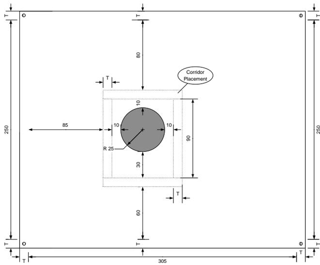
Fig. 25: Tunneling Ball Device topboard top view.
