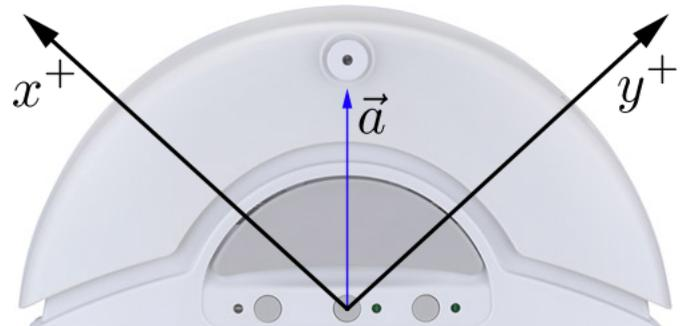
Fig. 2: Coordinate system for iRobot orientation with respect to gravity. The acceleration vector has positive and equal  $x$  and  $y$  components, indicating uphill orientation.
