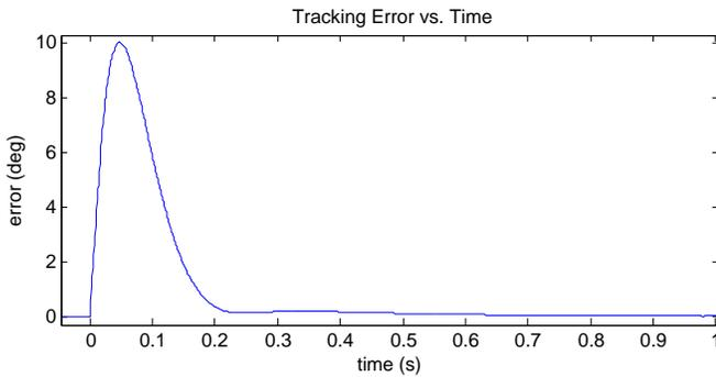
Fig. 13: Simulated error in disc position tracking via PID control. For times  $t < 0$ , the disc is in steady-state with  $\omega_0 = 4\text{rps}$ . For times  $t \geq 0$ , the desired position tracks a new rate of  $5\text{rps} \approx \omega_0 + \theta_{\max}/t_{\min}$ , and the PID controller adjusts to compensate.
