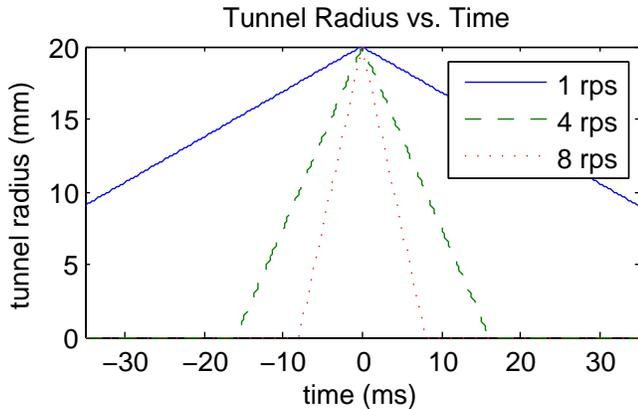
Fig. 14: Tunnel radius  $R_T(t)$  for different values of  $\omega_0$ . Motor constants substituted from the datasheet for a Maxon Re-35 motor [33].
