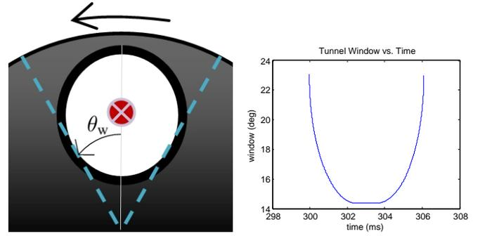
(a) Range through which a (b) Tunnel window as a ball nonzero tunnel exists,  $(-\theta_w, \theta_w)$ . passes through the disc.
