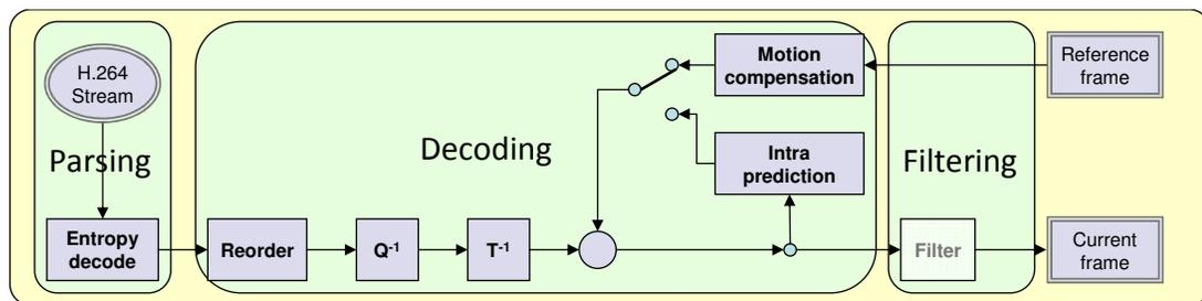
Figure 4.5: Block diagram of the H.264 decoder.
