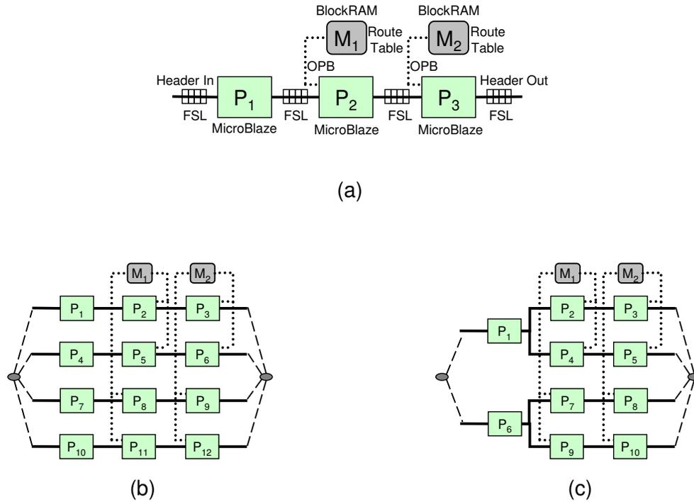
Figure 2.10: Different target architectures for IPv4 packet forwarding.
