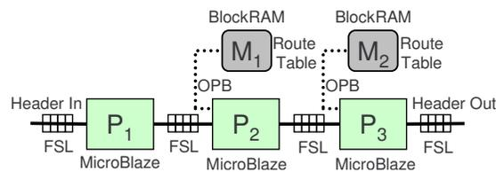
Figure 2.3: Architecture model of a soft multiprocessor composed of an array of 3 processors.
