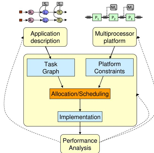
Figure 1.1: The Y-Chart approach for deploying concurrent applications.
