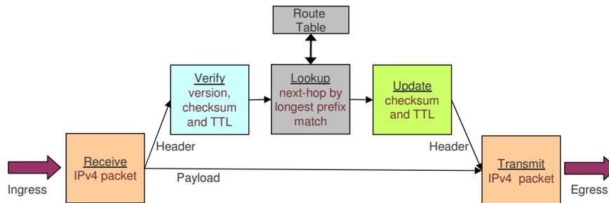
Figure 2.1: Block diagram of the data plane of the IPv4 packet forwarding application.
