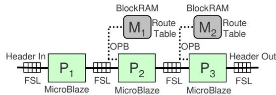
Figure 4.14: Architecture model of a soft multiprocessor composed of an array of 3 processors.
