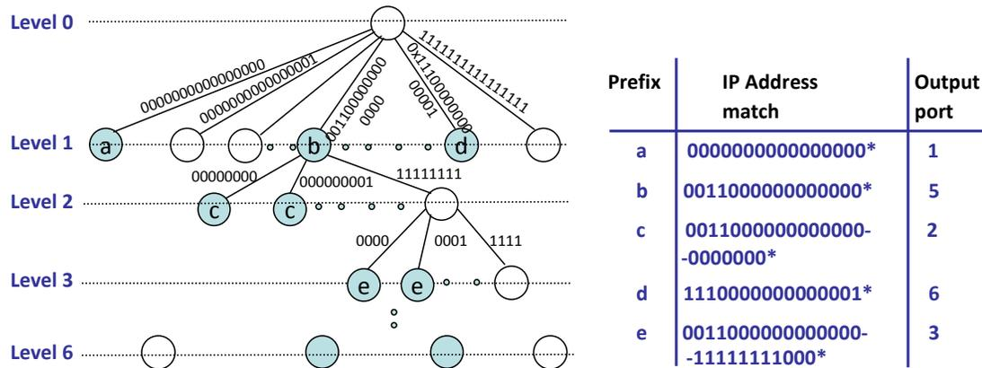
Figure 4.2: Example of a multi-bit trie with stride order (12 8 4 3 3 2) and the corresponding route table.
