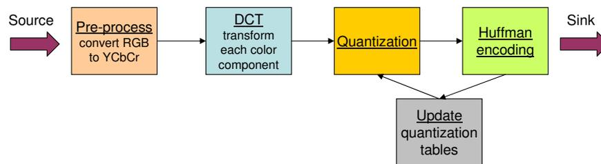
Figure 2.2: Block diagram of the Motion JPEG video encoding application.
