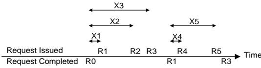
Figure 5: Intervals between Issuance of I/O Requests and Most Recent Request Completion.
