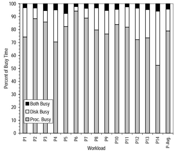
Figure 3: Disk and Processor Busy Time.
