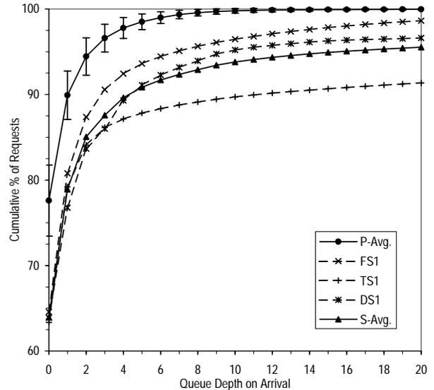
Figure 8: Distribution of Queue Depth on Arrival. Bars indicate standard deviation.
