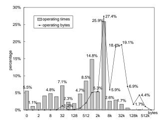
Figure 4: Write File System Call Block Size vs. Access Times and Total Bytes Written
