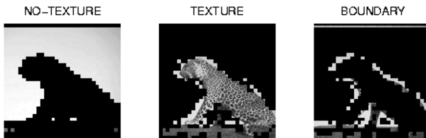
Fig. 2. Detection of non-textured regions, textured regions and boundary elements on a Cheeta image. Local windows, of size 4 \times 4 are categorized into the 3 classes. Boundary elements correspond to both intensity-edges as well as textured-edges. Windows are labeled as boundary if they have a low histogram cross-correlation figure in both resolutions of analysis. We note the importance of detecting the no-texture region as a step which enables to focus further attention to the more-interesting, textured regions of the image - in this example, focusing the attention on the animal figure. The textured region extracts the entire cheeta, as well as the grass. Further, more detailed investigation on the extracted textured regions (using blob-finding or repetitive-pattern region-growing, for example, both schemes which will be described below), will enable a refined distinction between the cheeta and its surrounding. We note that the extraction of boundary information unified with textured-region information, helps eliminate the confusion between the true animal boundary and the many edges which exist within the cheeta's textured body (classic edge-finding schemes will detect all the circular edges as well).
