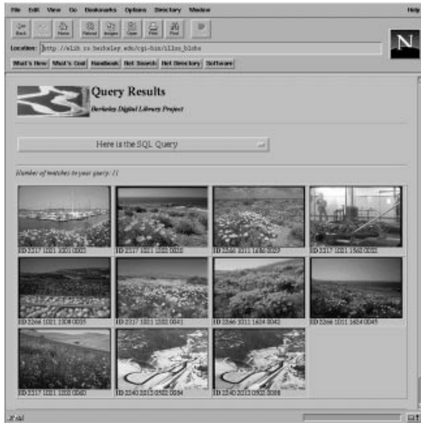
Fig. 5. Querying the Cypress database for images that contain a large number of small yellow blobs and a horizon yields scenic views of fields of flowers. The horizon is obtained by searching in from each boundary of the image for a blue region, extending to the boundary, that does not curve very sharply. In this case, the combination of spatial and color queries yields a query that encapsulates content surprisingly well. While the correlation between object type and query is fortuitous, and relevant only in the context of the particular database, it is clear that the combination of spatial and chromatic information in the query yields a more powerful content query than color alone. In particular, the language of blobs is a powerful and useful early cue to content. Note that the ordering of the images in response to the query (as presented in this figure) is arbitrary. No relative ranking is performed.
