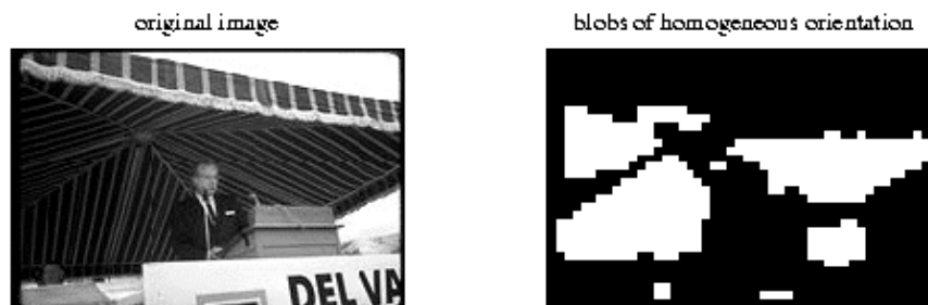
Fig. 11. The homogeneously oriented regions in the striped canopy in the image on the left show up as distinct blobs in the result of the second grouping strategy, shown on the right. (The color/texture separation was equal to one everywhere, thus defining the entire image as a potential area of interest.)
