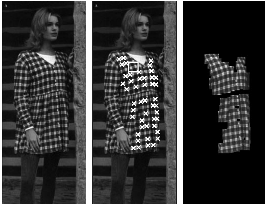
Fig. 3. A textile image. The original image is shown on the left, and the center image shows the initial patches found. The crosses are the locations of units grouped together. The image on the right shows the segmented region is displayed. Notice that the rectangle includes two units in the actual pattern. This is due to the inherent ambiguity in defining a repeating unit - 2 tiles together still repeat to form a pattern.
